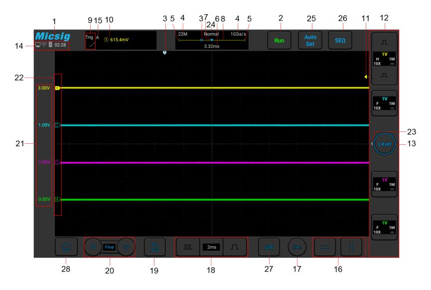
Figure 2-6 Oscilloscope Interface Display
