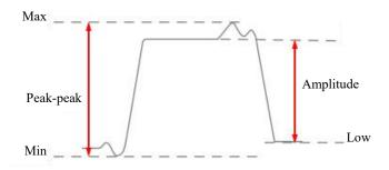
Figure 6-7 Voltage Measurement
