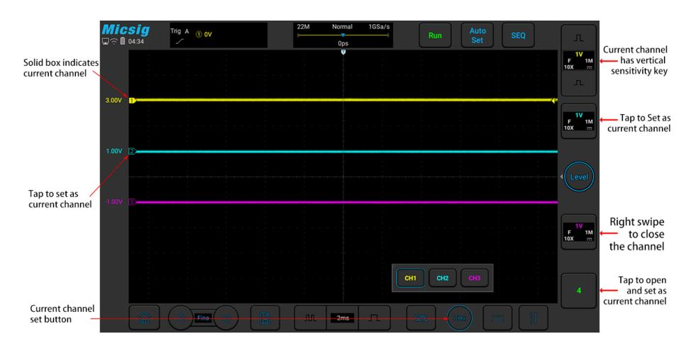
Figure 4-4 Channel Open, Close and Switching
