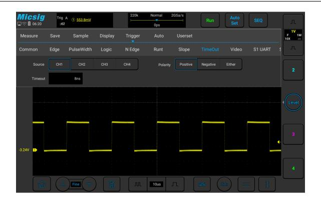
Figure 5-29 Time-out Trigger
