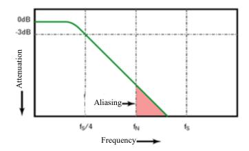
Figure 10-3 Sampling Rate and Oscilloscope Bandwidth
