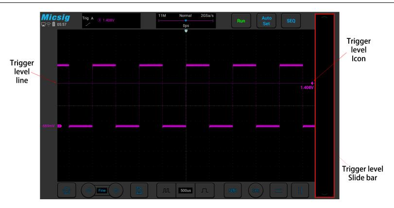
Figure 5-8 Trigger Level
