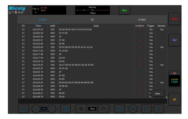
Figure 11-25 I2C Text Interface
