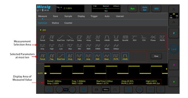
Figure 6-1 Automatic Measurement Menu
