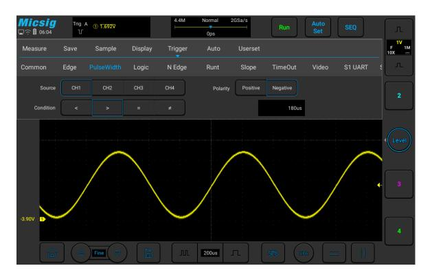
Figure 5-15 Negative Polarity Pulse Level Flip
