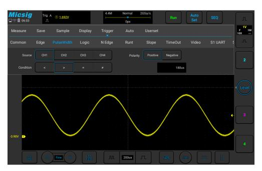
Figure 5-14 Pulse Width Trigger Setting Menu
