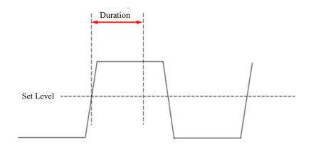
Figure 5-28 Timeout Trigger Schematics
