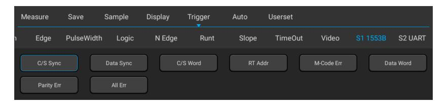
Figure 11-31 1553B Trigger Mode Configuration Menu
