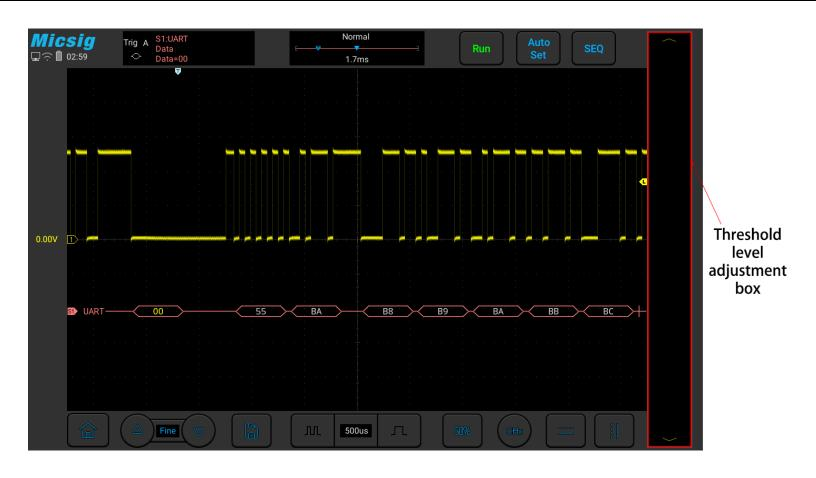
Figure 11-7 UART Decode Level Adjustment
