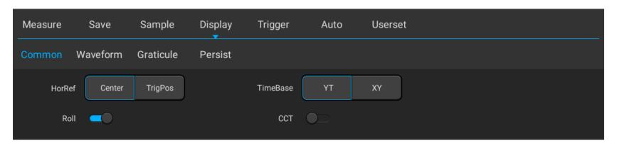
Figure 3-7 Roll Mode On/Off
