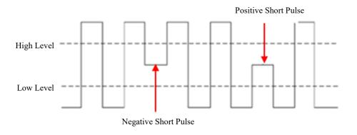
Figure 5-24 Runt Trigger
