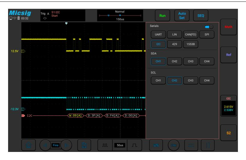
Figure 11-22 I2C Bus Configuration Menu
