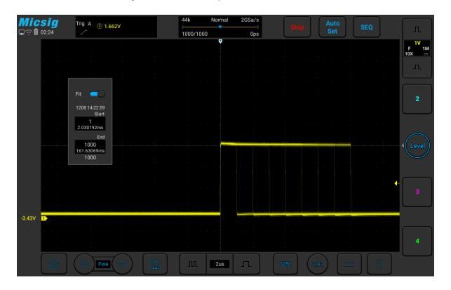
Figure 10-13 Segmented storage fitting view
