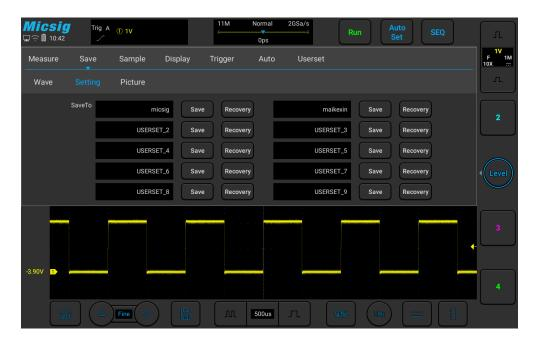
Figure 7-7 oscilloscope setting save
