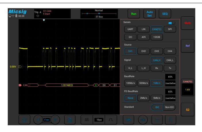
Figure 11-14 CAN(FD) Bus Configuration Menu
