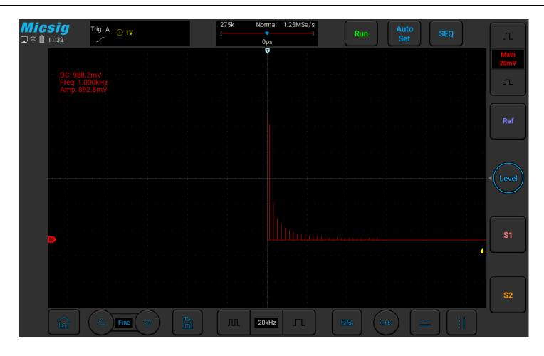
Figure 8-4 Spectrum Amplitude as V-Hz
