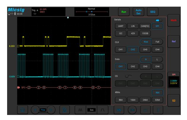
Figure 11-18 SPI Bus Configuration Menu
