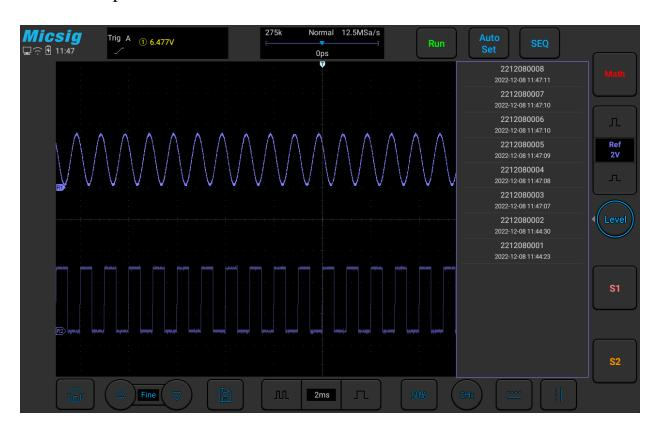
Figure 8-7 Restore Reference Waveform
