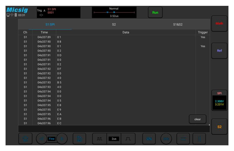
Figure 11-21 SPI Text Interface
