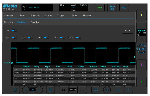
Figure 6-8 Frequency Meter Measurement Menu Open
