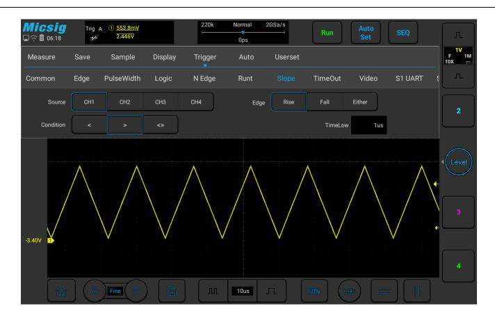
Figure 5-27 Slope Trigger Setting Menu
