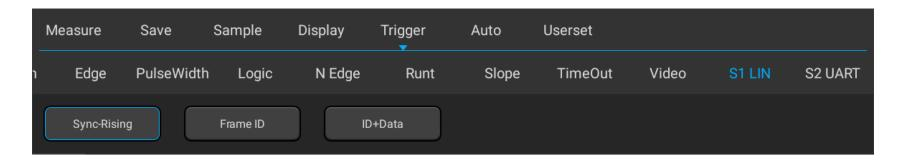
Figure 11-11 LIN Trigger Mode Configuration Menu
