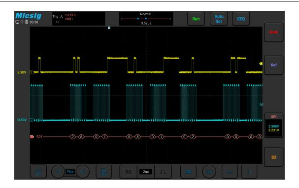
Figure 11-20 SPI Graphic Interface
