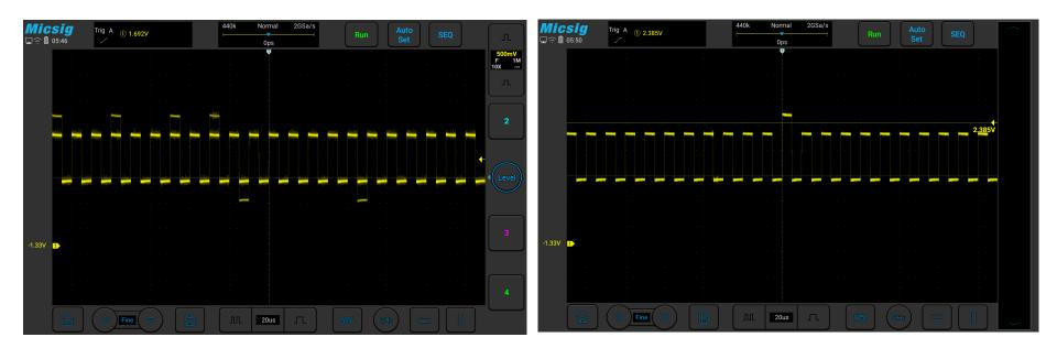
Figure 5-3 Abnormal Signal in Periodic Signals
