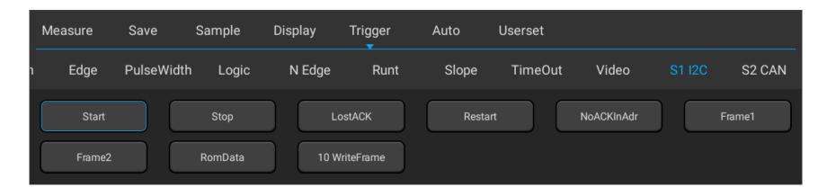
Figure 11-23 I2C Trigger Mode Configuration Menu
