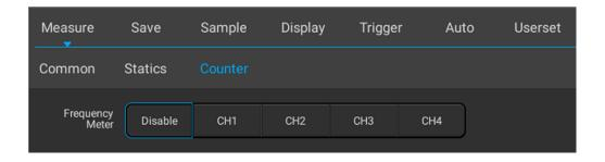
Figure 6-9 Frequency Meter Measurement Menu Open
