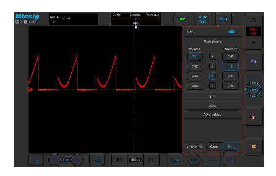
Figure 8-1 MATH Channel Waveform
