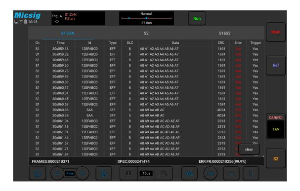
Figure 11-17 CAN Text Interface
