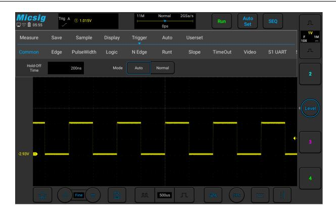
Figure 5-5 Oscilloscope Trigger Mode Setting
