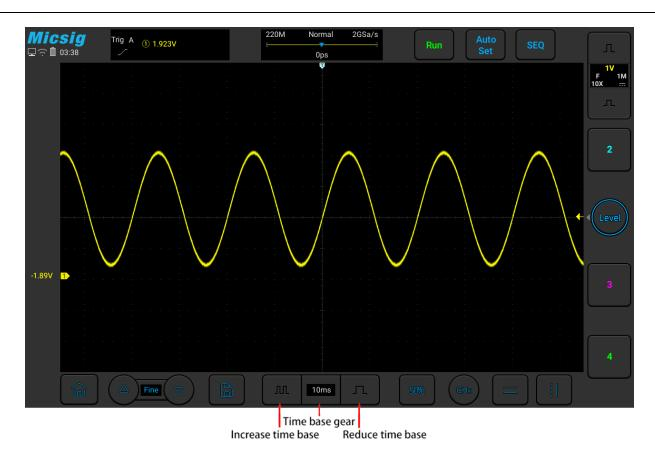
Figure 3-3 Adjust the Horizontal Time Base
