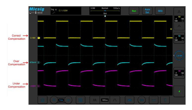
Figure 2-15 Probe Compensation
