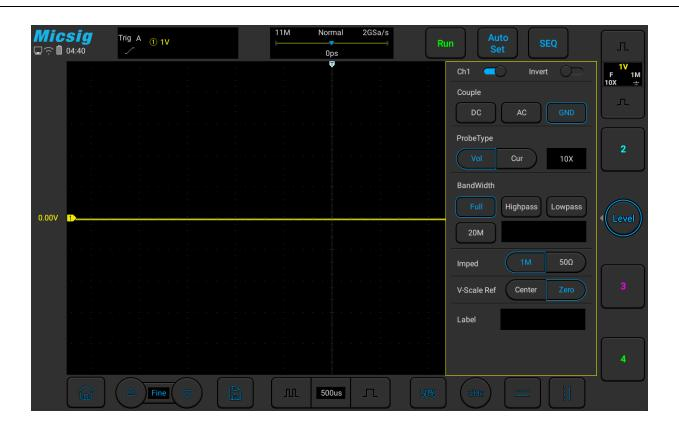
Figure 4-9 GND Coupling
