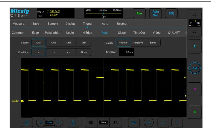
Figure 5-25 Runt Trigger Setting Menu
