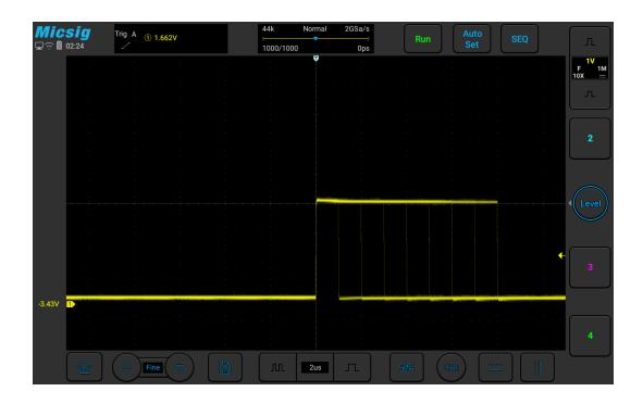
Figure 10-11 Segmented memory waveform acquisition
