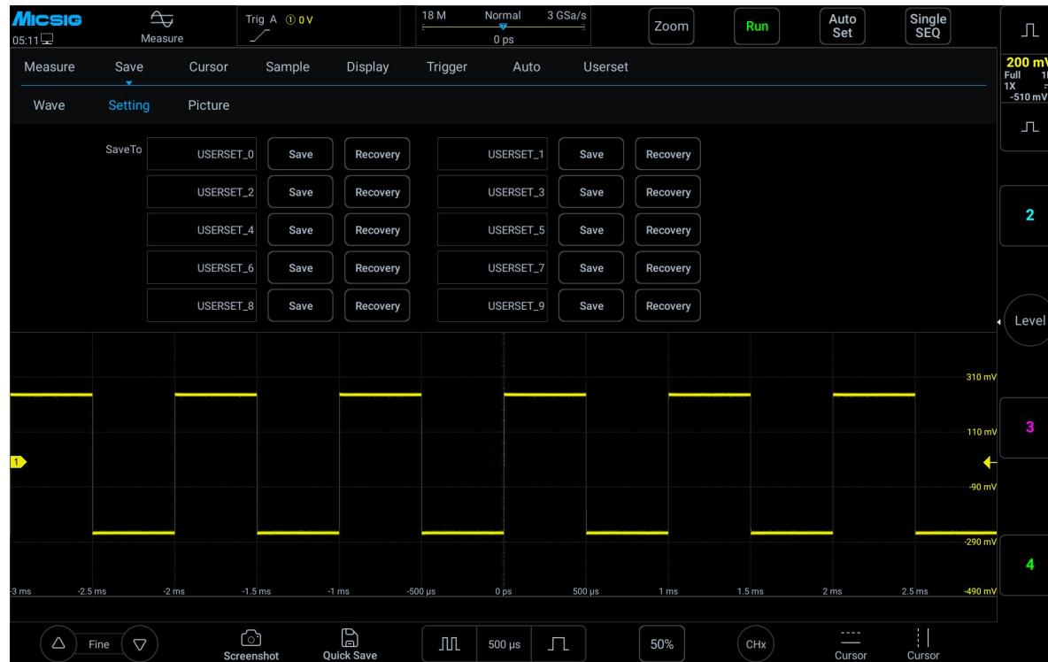
Figure 7-7 oscilloscope setting save
