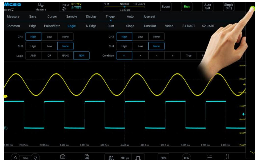
Figure 5-22 Trigger Level Adjustment
