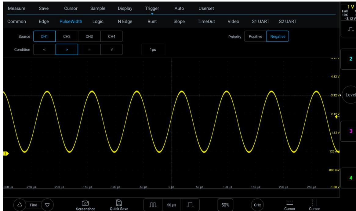
Figure 5-15 Negative Polarity Pulse Level Flip
