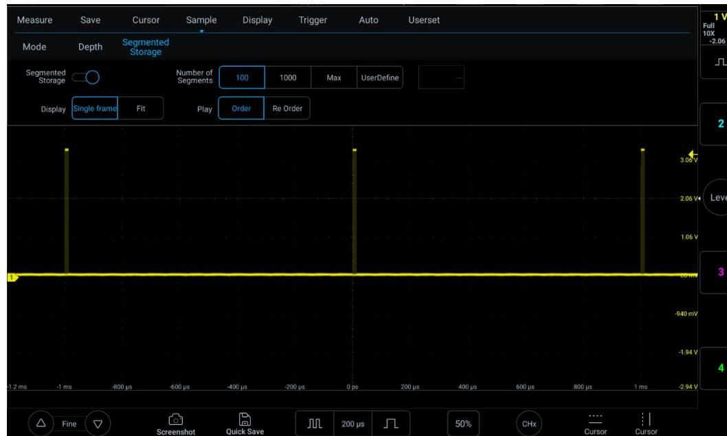
Figure 10-11 Segmented storage waveform acquisition
