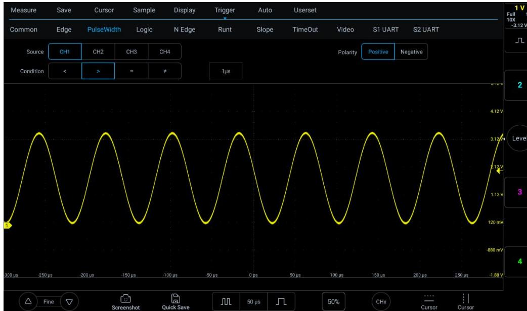
Figure 5-14 Pulse Width Trigger Setting Menu
