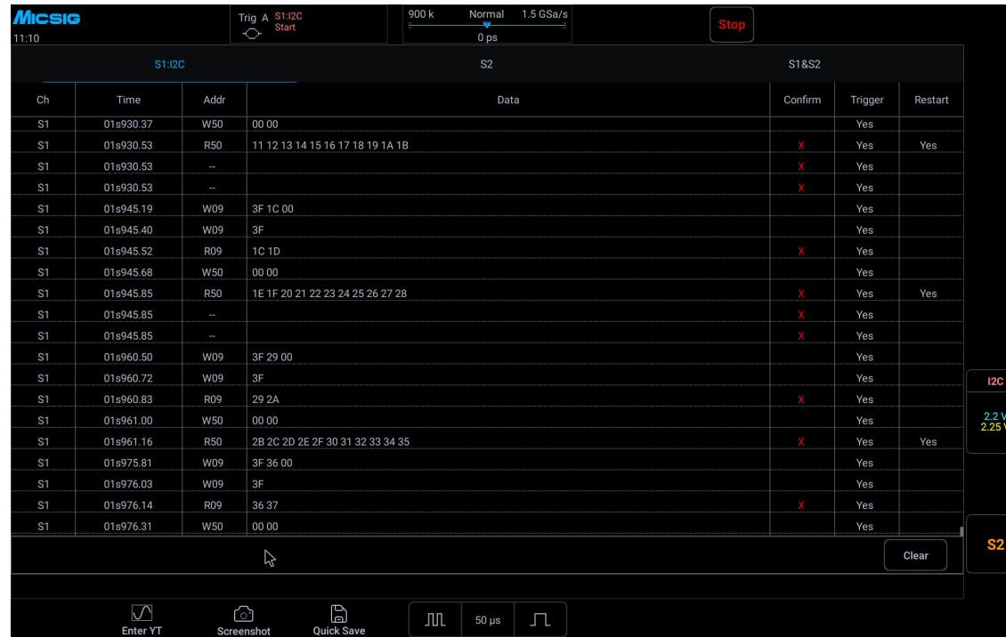
Figure 11-25 I<sup>2</sup>C Text Interface
