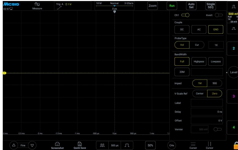
Figure 4-9 GND Coupling
