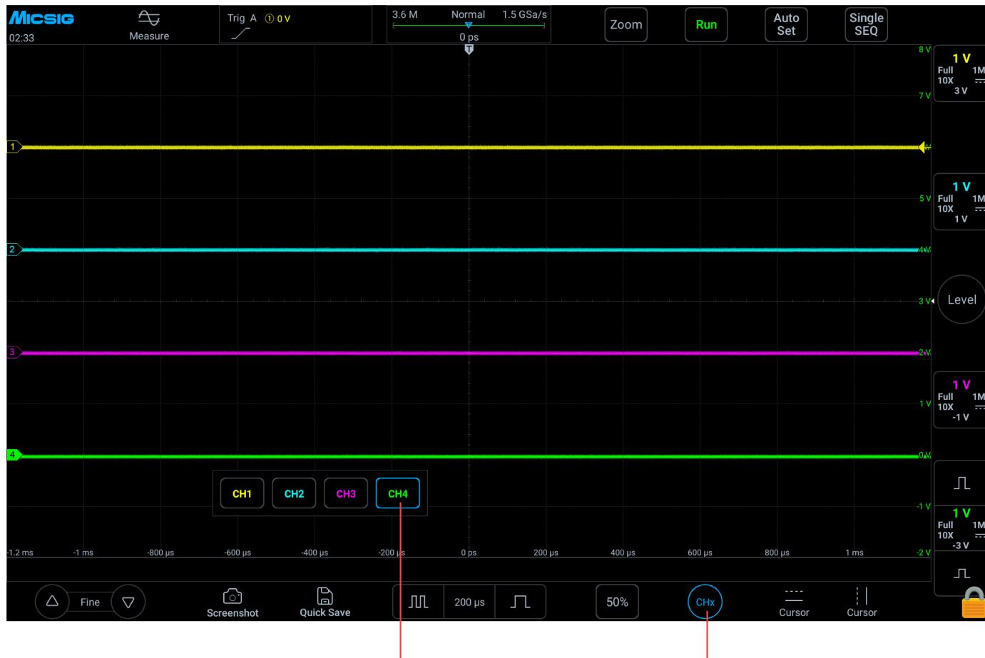
Figure 4-5 Using the Current Channel Selection Button
