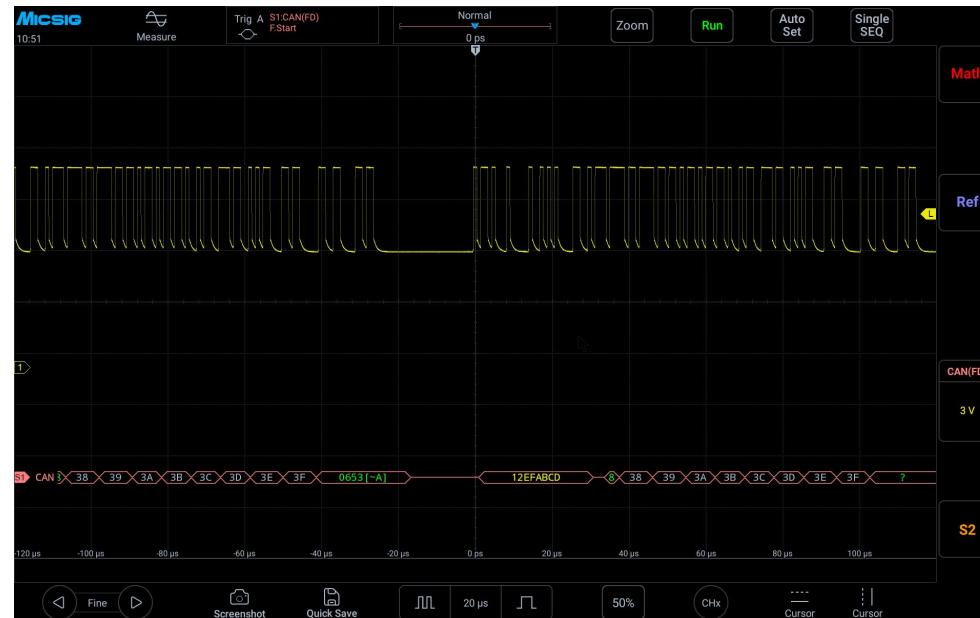
Figure 11-16 CAN bus decode interface
