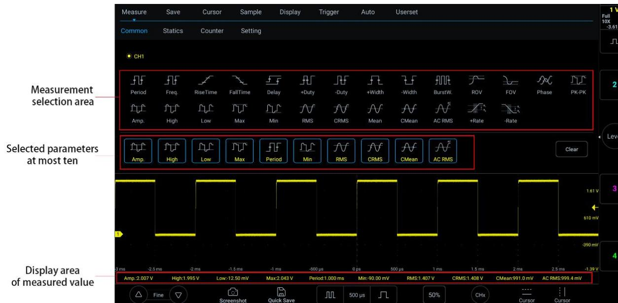
Figure 6-1 Automatic Measurement Menu
