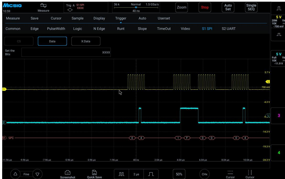
Figure 11-20 SPI bus decode interface
