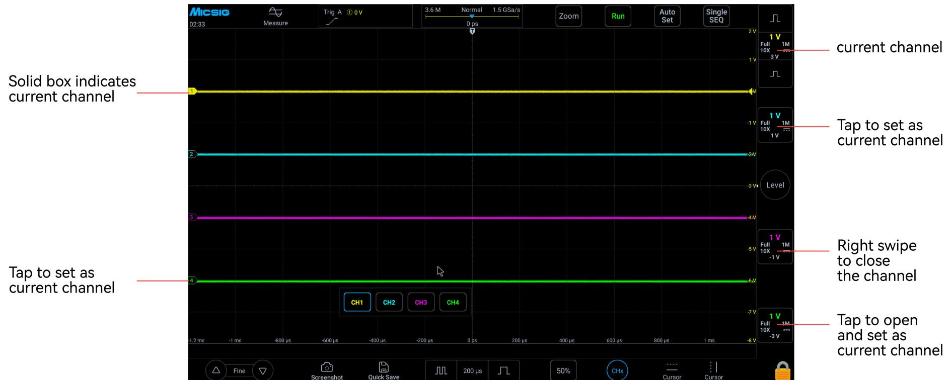
Figure 4-4 Channel Open, Close and Switching
