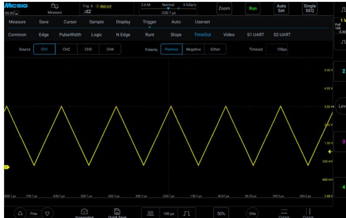
Figure 5-29 Time-out Trigger
