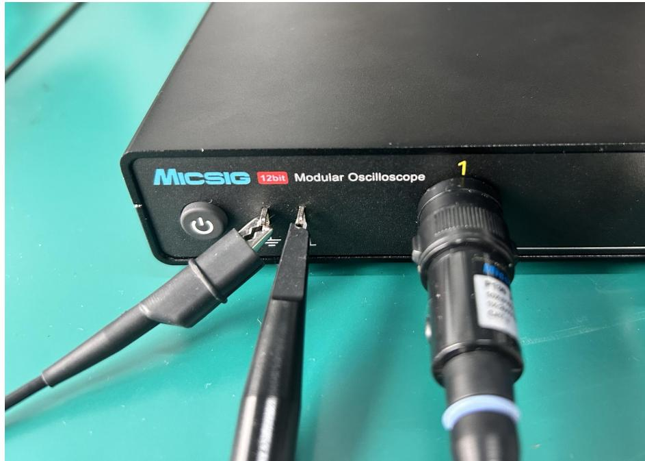
Figure 2-12 Probe Connection
