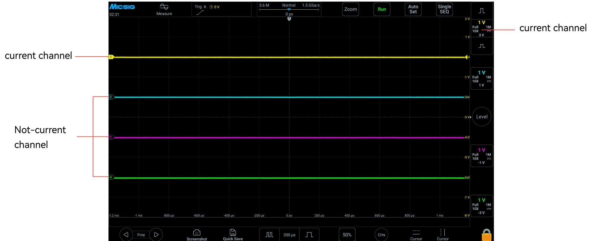
Figure 4-2 Current Channel and Non-Current Channel
