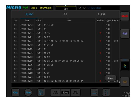
Figure 12-25 I2C Text Interface
