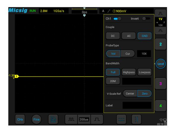
Figure 5-9 GND Coupling
