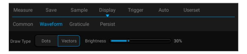
Figure 10-2 Waveform Display Menu
