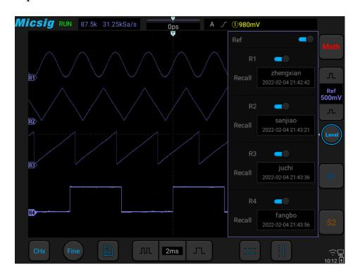
Figure 9-7 Restore Reference Waveform
