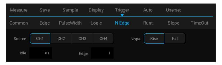
Figure 6-12 Edge Trigger Setting Menu
