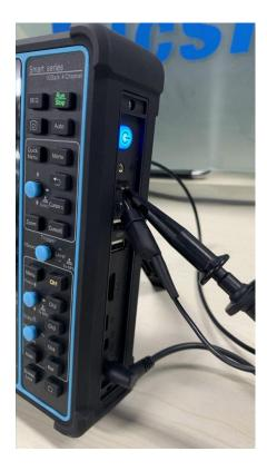
Figure 2-13 Probe Connection
