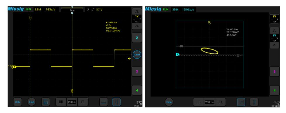
Figure 7-12 Cursor Measurement Pulse Width
