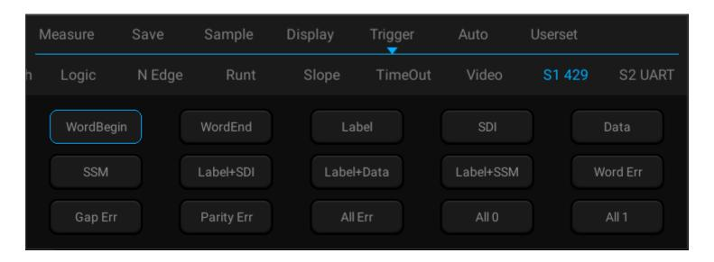
Figure 12-27 ARINC429 Trigger Mode Configuration Menu
