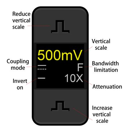
Figure 5-3 Channel Display Interface
