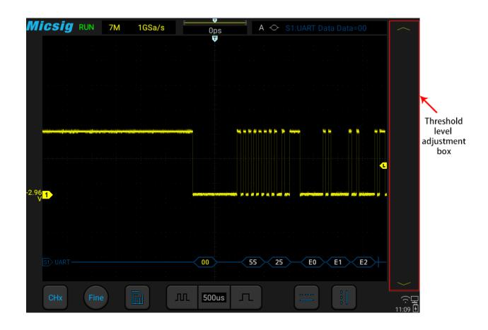
Figure 12-7 UART Decode Level Adjustment
