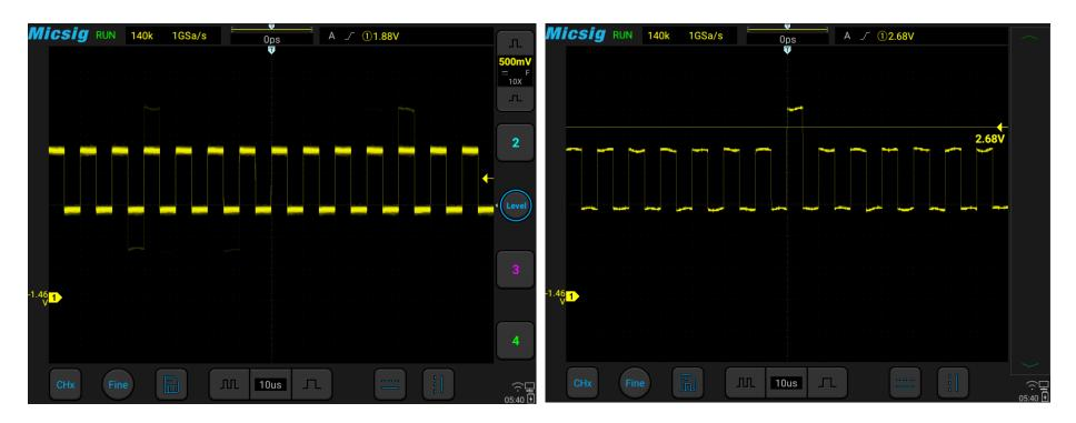
Figure 6-3 Abnormal Signal in Periodic Signals
