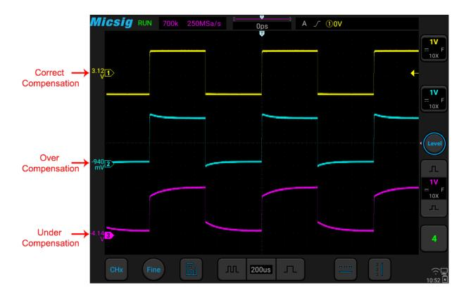
Figure 2-14 Probe Compensation
