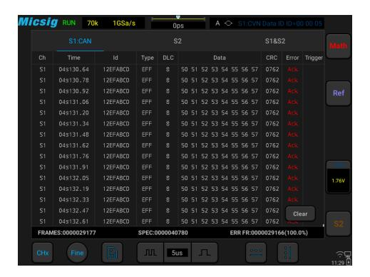
Figure 12-17 CAN Text Interface
