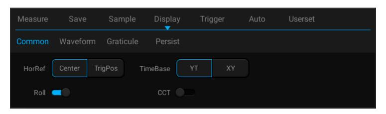
Figure 4-7 Roll Mode On/Off
