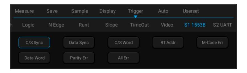
Figure 12-31 1553B Trigger Mode Configuration Menu
