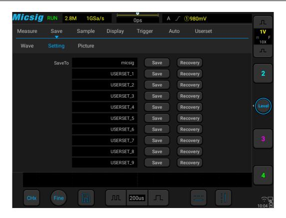
Figure 8-7 oscilloscope setting save
