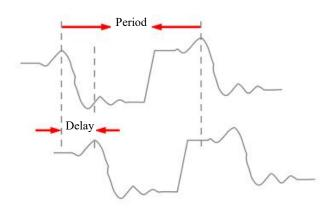
Figure 7-6 Phase Measurement Schematics
