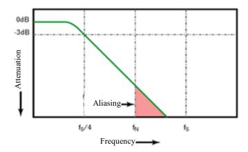
Figure 11-3 Sampling Rate and Oscilloscope Bandwidth
