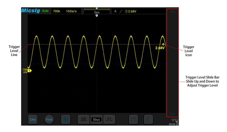
Figure 6-8 Trigger Level
