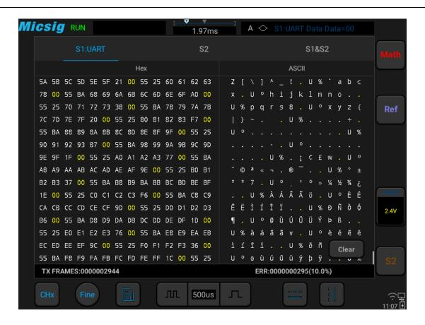
Figure 12-2 Bus Decode Text Mode
