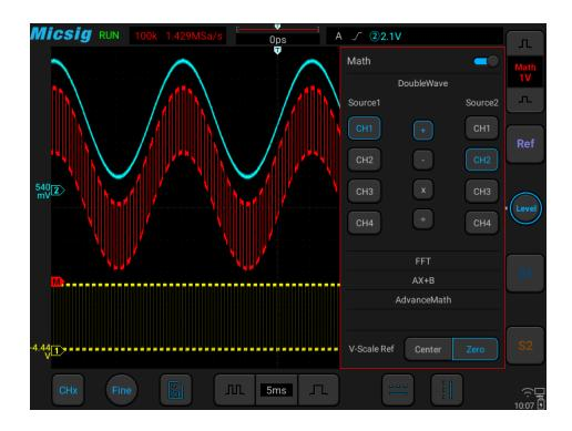
Figure 9-2 Mathematical Operation of CH1 adding CH2
