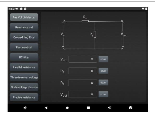
Figure 13-10 Electronic Calculation Tool Function
