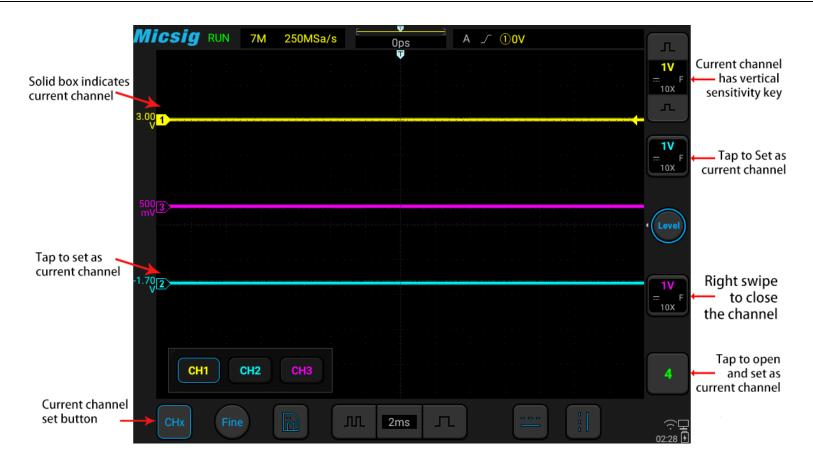
Figure 5-4 Channel Open, Close and Switching
