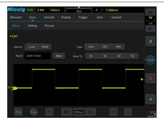
Figure 8-5 Save CH1 Reference Waveform Interface
