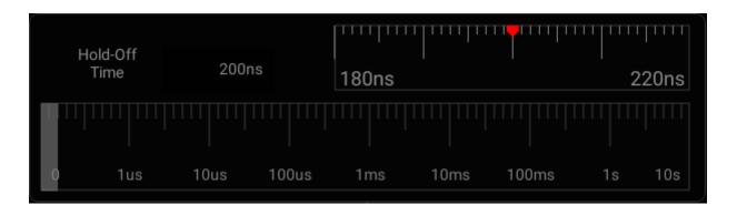
Figure 3-2 Trigger hold-off time
