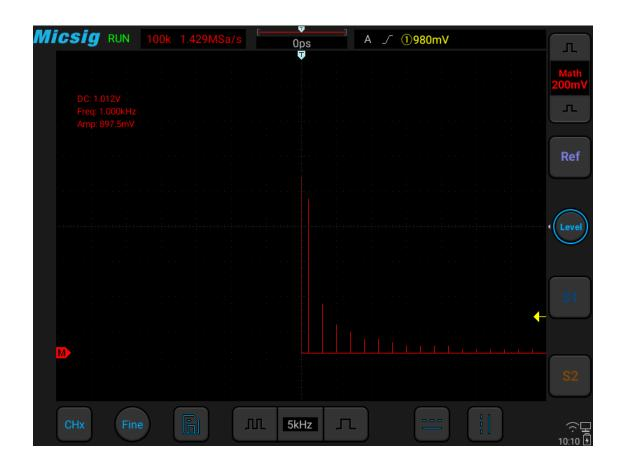
Figure 9-4 Spectrum Amplitude as V-Hz
