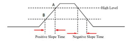
Figure 6-26 Positive/Negative Slope Time
