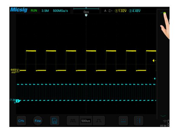
Figure 6-22 Trigger Level Adjustment
