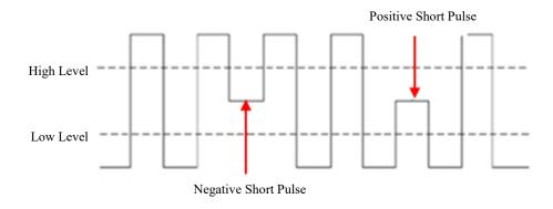
Figure 6-24 Runt Trigger
