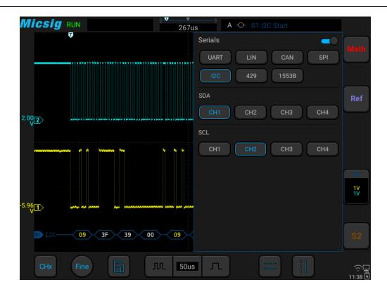
Figure 12-22 I2C Bus Configuration Menu
