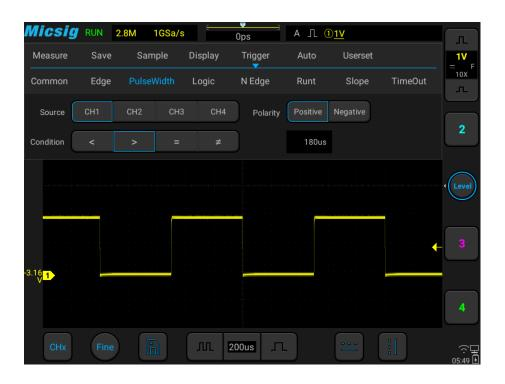
Figure 6-14 Pulse Width Trigger Setting Menu
