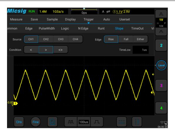
Figure 6-27 Slope Trigger Setting Menu
