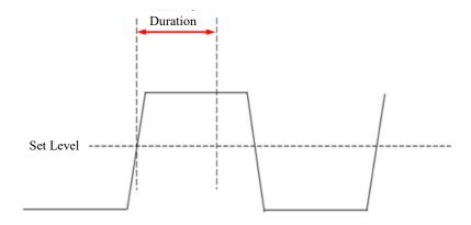
Figure 6-28 Timeout Trigger Schematics
