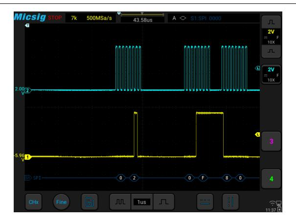
Figure 12-20 SPI Graphic Interface
