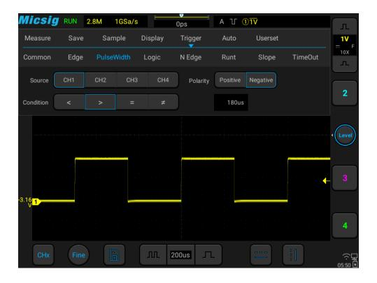
Figure 6-15 Negative Polarity Pulse Level Flip
