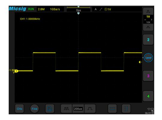
Figure 7-9 Frequency Meter Measurement
