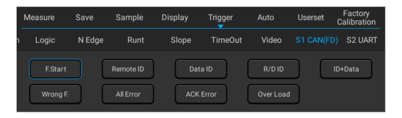
Figure 12-15 CAN Trigger Mode Configuration Menu
