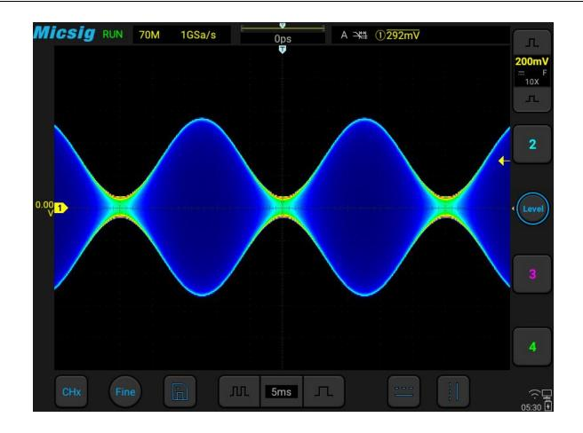
Figure 10-5 Color Temperature Open Mode
