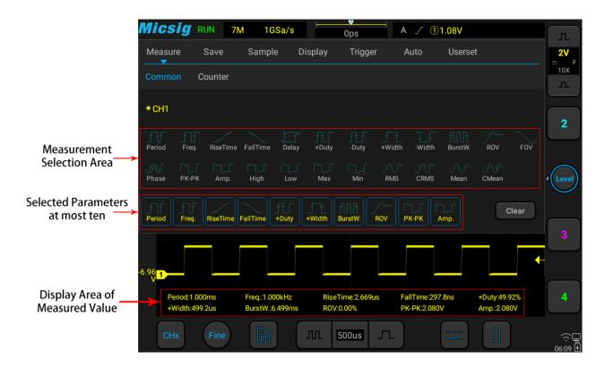
Figure 7-1 Automatic Measurement Menu
