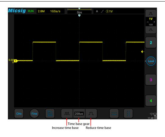
Figure 4-3 Adjust the Horizontal Time Base
