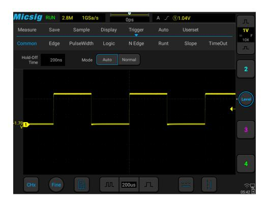
Figure 6-5 Oscilloscope Trigger Mode Setting
