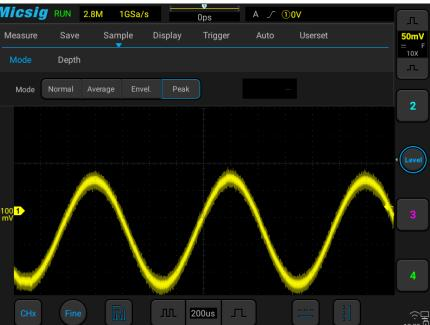
Figure 11-5 Sine Wave with Burr
