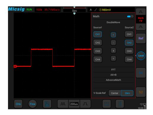
Figure 9-1 MATH Channel Waveform
