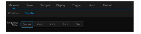
Figure 7-8 Frequency Meter Measurement Menu Open
