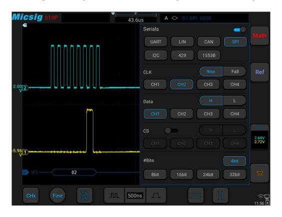
Figure 12-18 SPI Bus Configuration Menu
