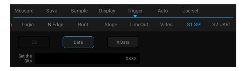
Figure 12-19 SPI Trigger Mode Configuration Menu
