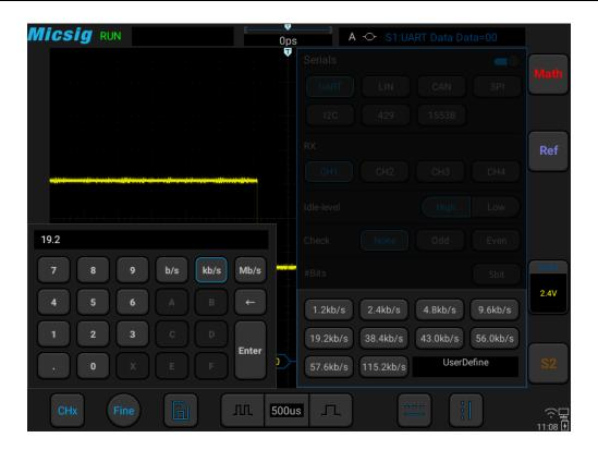
Figure 12-5 Baud Rate Default Setting
