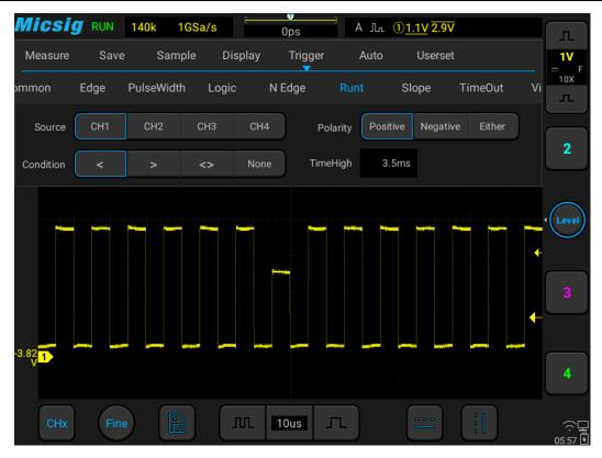
Figure 6-25 Runt Trigger Setting Menu
