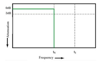
Figure 11-2 Theoretical Brick-Wall Frequency Response
