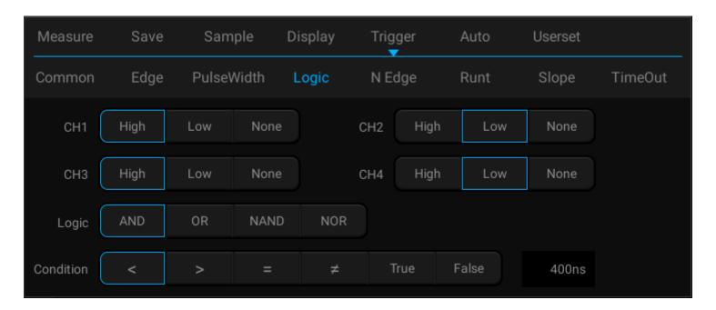
Figure 6-21 Logic Trigger Setting Menu
