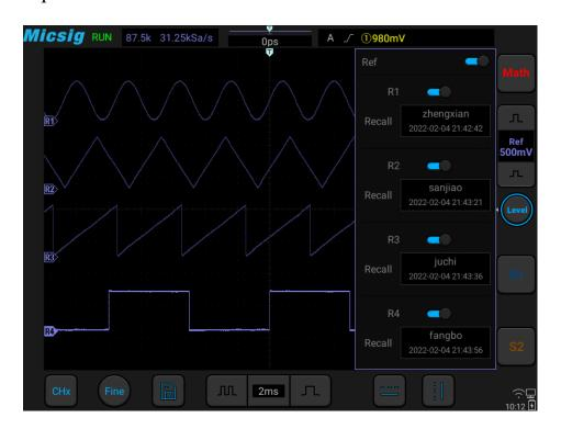
Figure 9-7 Restore Reference Waveform
