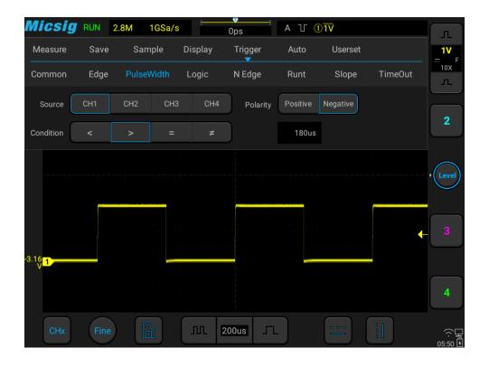
Figure 6-15 Negative Polarity Pulse Level Flip
