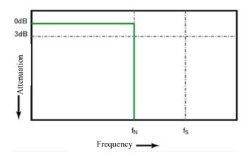
Figure 11-2 Theoretical Brick-Wall Frequency Response
