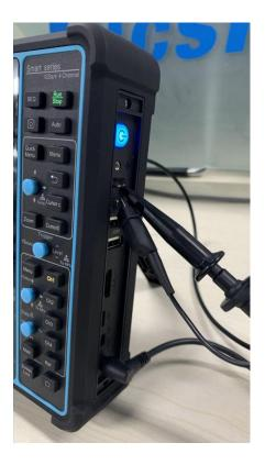
Figure 2-13 Probe Connection
