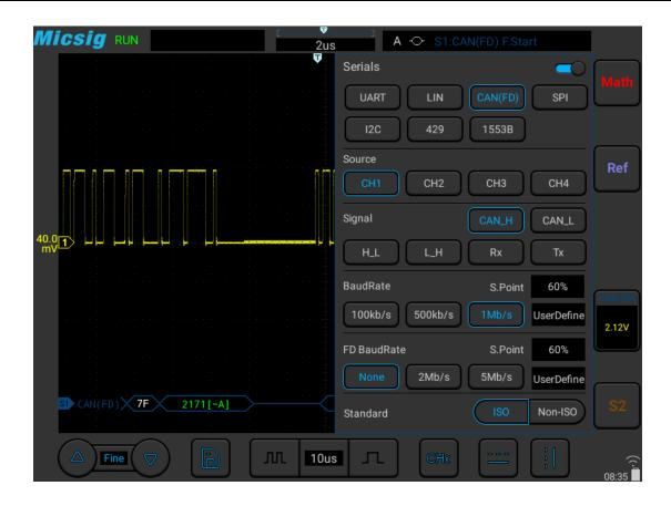
Figure 12-14 CAN / CAN FD Bus Configuration Menu
