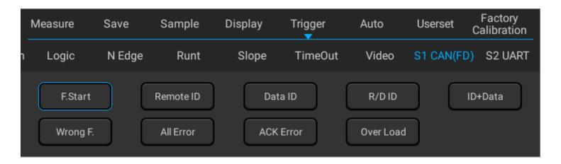
Figure 12-15 CAN Trigger Mode Configuration Menu
