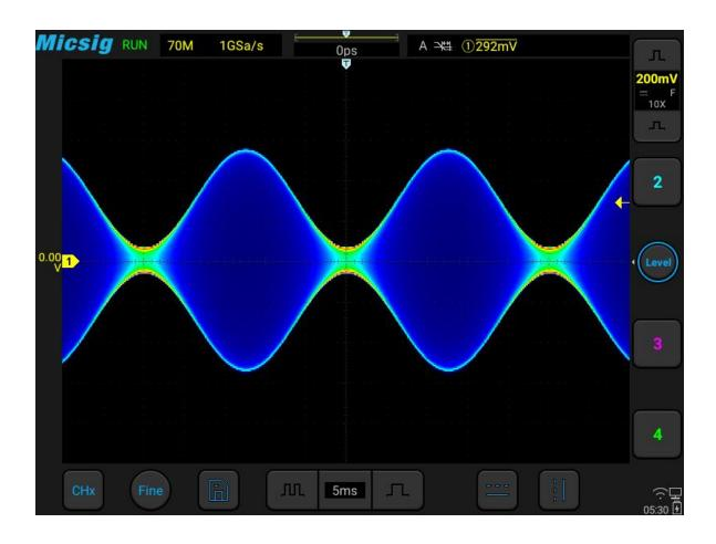
Figure 10-5 Color Temperature Open Mode
