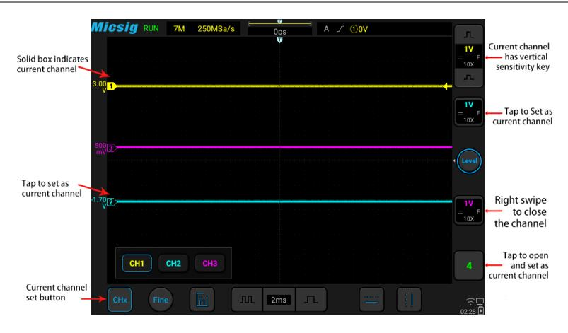
Figure 5-4 Channel Open, Close and Switching
