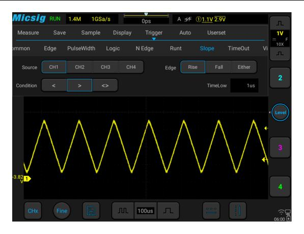
Figure 6-27 Slope Trigger Setting Menu
