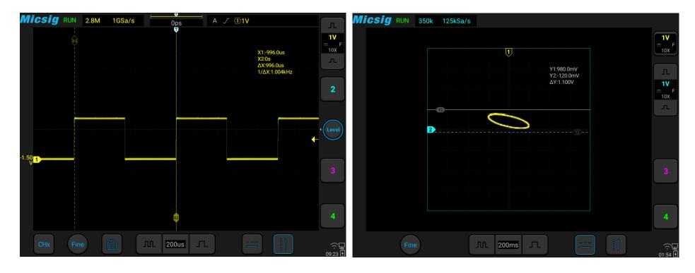
Figure 7-18 Cursor Measurement Pulse Width
