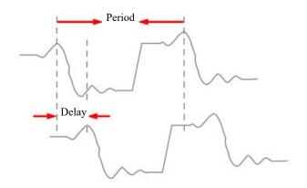
Figure 7-6 Phase Measurement Schematics
