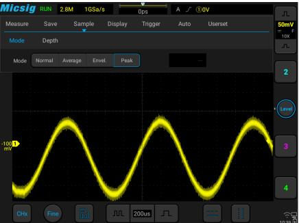
Figure 11-5 Sine Wave with Burr
