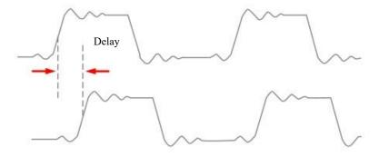
Figure 7-5 Delay Measurement Schematics
