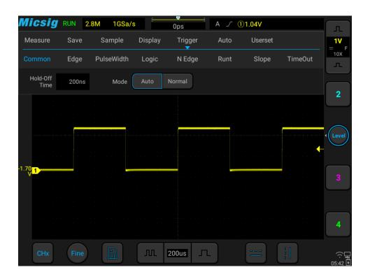
Figure 6-5 Oscilloscope Trigger Mode Setting
