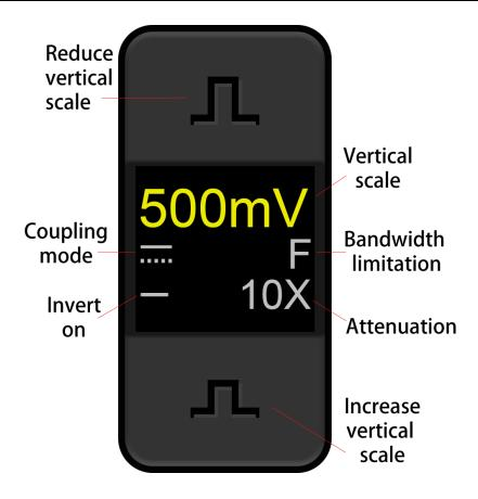
Figure 5-3 Channel Display Interface
