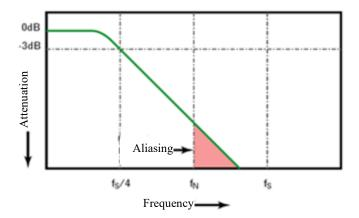
Figure 11-3 Sampling Rate and Oscilloscope Bandwidth
