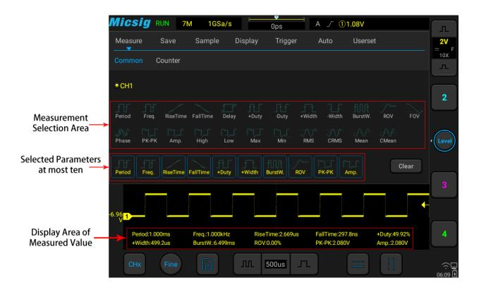
Figure 7-1 Automatic Measurement Menu
