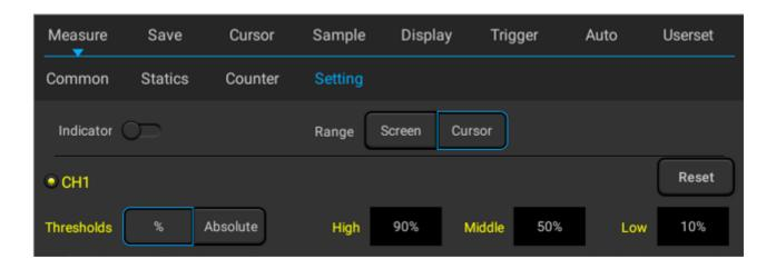
Figure 7-12 Measure Thresholds
