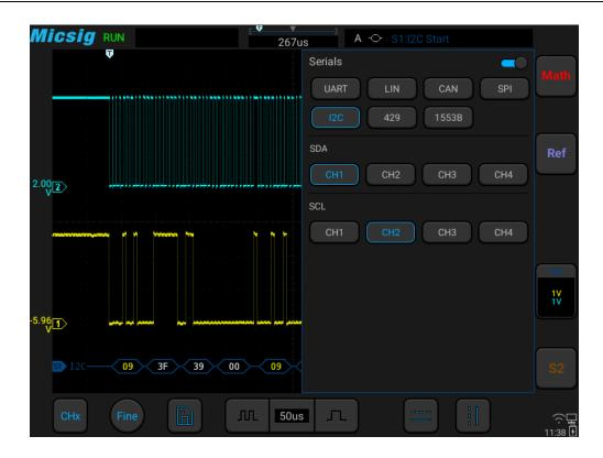
Figure 12-22 I2C Bus Configuration Menu
