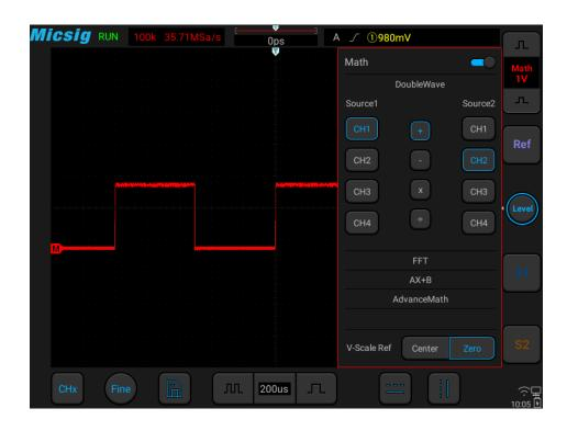
Figure 9-1 MATH Channel Waveform
