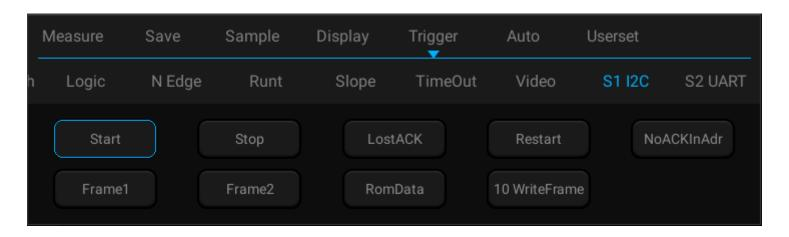
Figure 12-23 I2C Trigger Mode Configuration Menu
