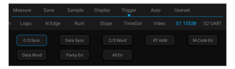
Figure 12-31 1553B Trigger Mode Configuration Menu
