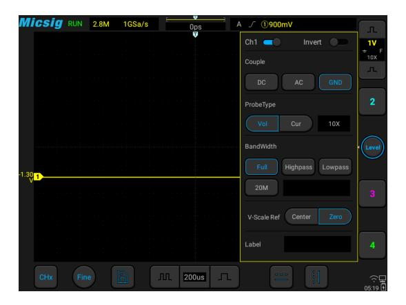
Figure 5-9 GND Coupling
