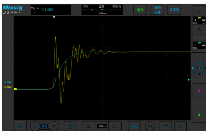
▲ Vgs signal at SiC conduction moment
