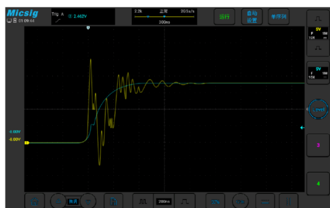
▲ Vgs signal at SiC conduction moment
