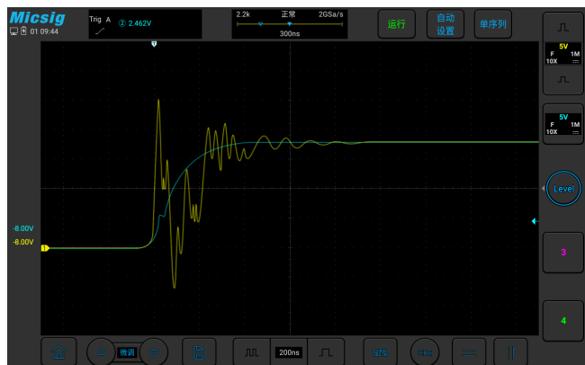
Yellow: Differential Probe Blue: SigOFIT Optical-fiber Isolated Probe
