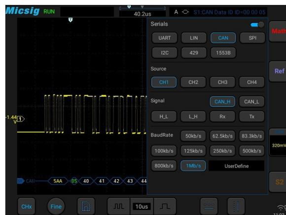
**▲ Serial Bus Decoding and Analysis**
