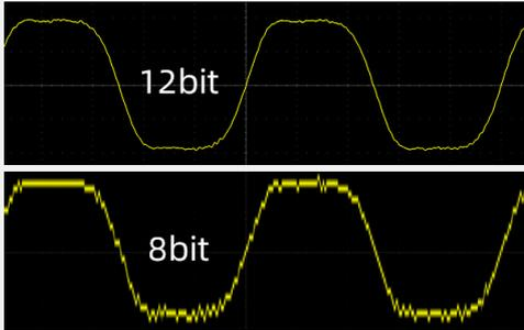
► MHO series has 12 bit high-resolution ADC with a quantization level of up to 4096, it's 16 times that of traditional 8-bit ADC, present unmatched waveform details.
