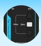
CP503B/CP1003B: Press the Zero button "□", light on, the probe will carry out Degaussing and Zero setting
