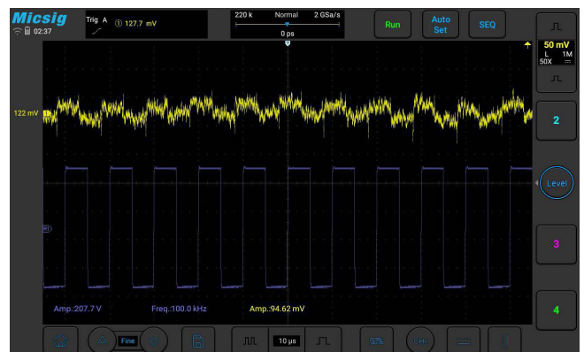
CH1: @ 100kHz, 207.7V, output common mode signal amplitude 94.62mV, CMRR > -70dB
