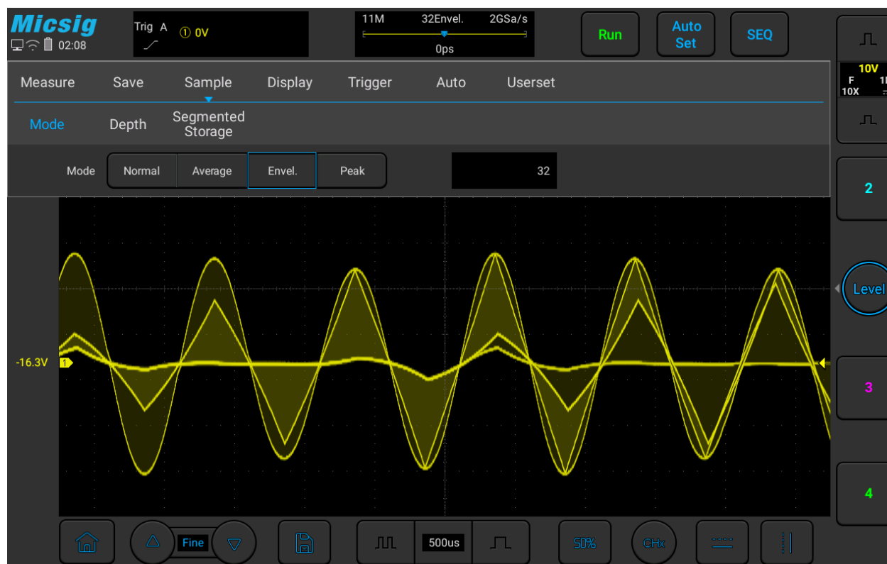
Figure 10-8 AM Signal in Envelope Sampling Mode (32)
