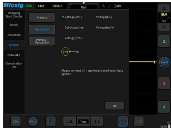
▲ The ignition system of a car is usually composed of primary and secondary coils and spark plugs. Can test both Primary and Secondary ignition signals, to find out possible malfunction.
