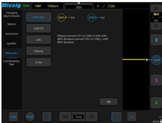
▲ SATO is capable of acquiring and decoding CAN High /CAN Low, CAN FD, LIN, FlexRay, and K line signals, delivers professional Network communication tests on vehicles.
