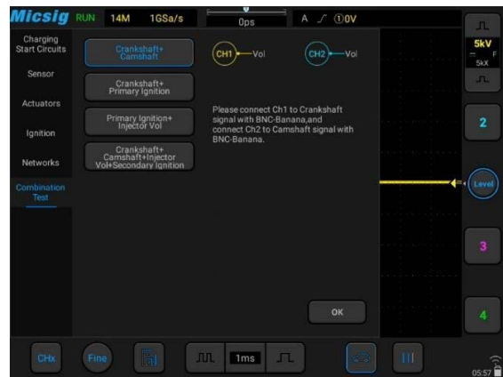
▲ The electronic faults can be complicated, by comparing the collected various waveforms, users judge faults by analyzing the timing and quantitative relationships between waveforms.
