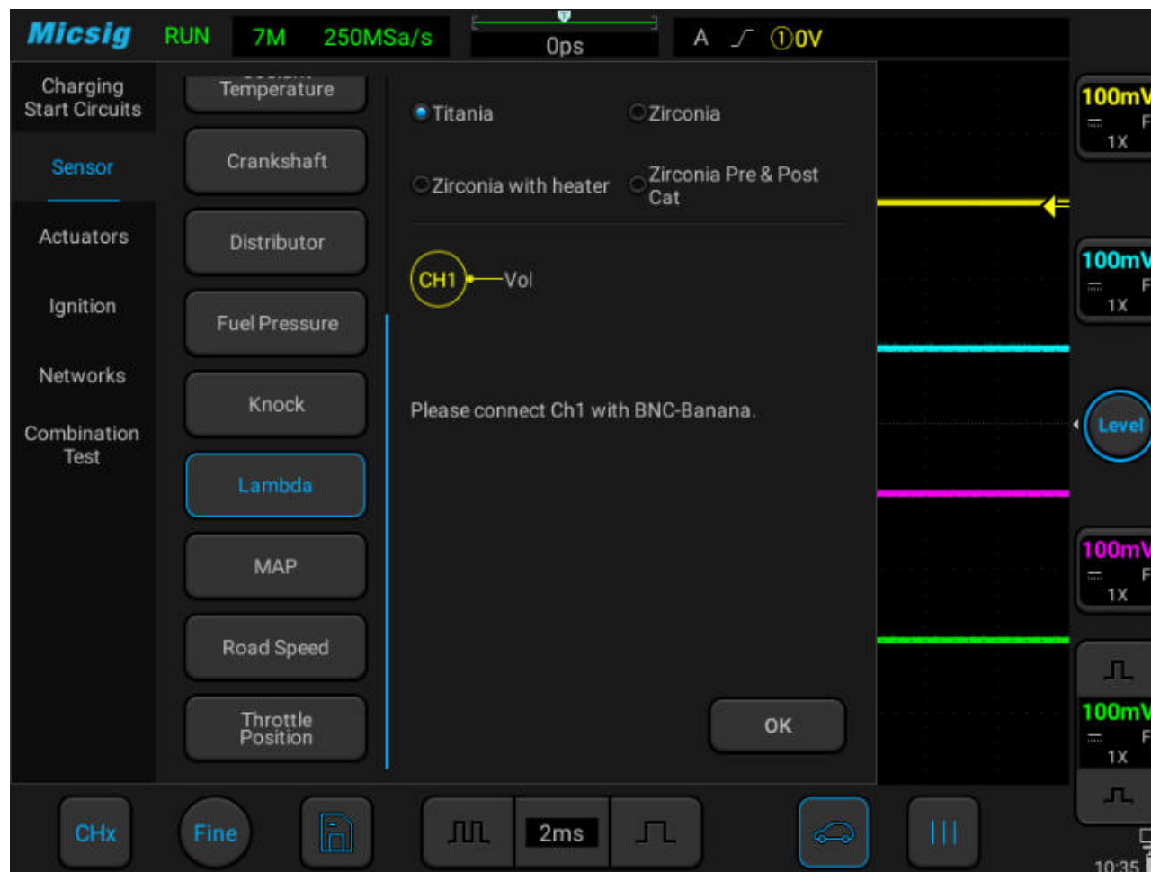
Figure 3-20 Lambda (oxygen sensor) test
