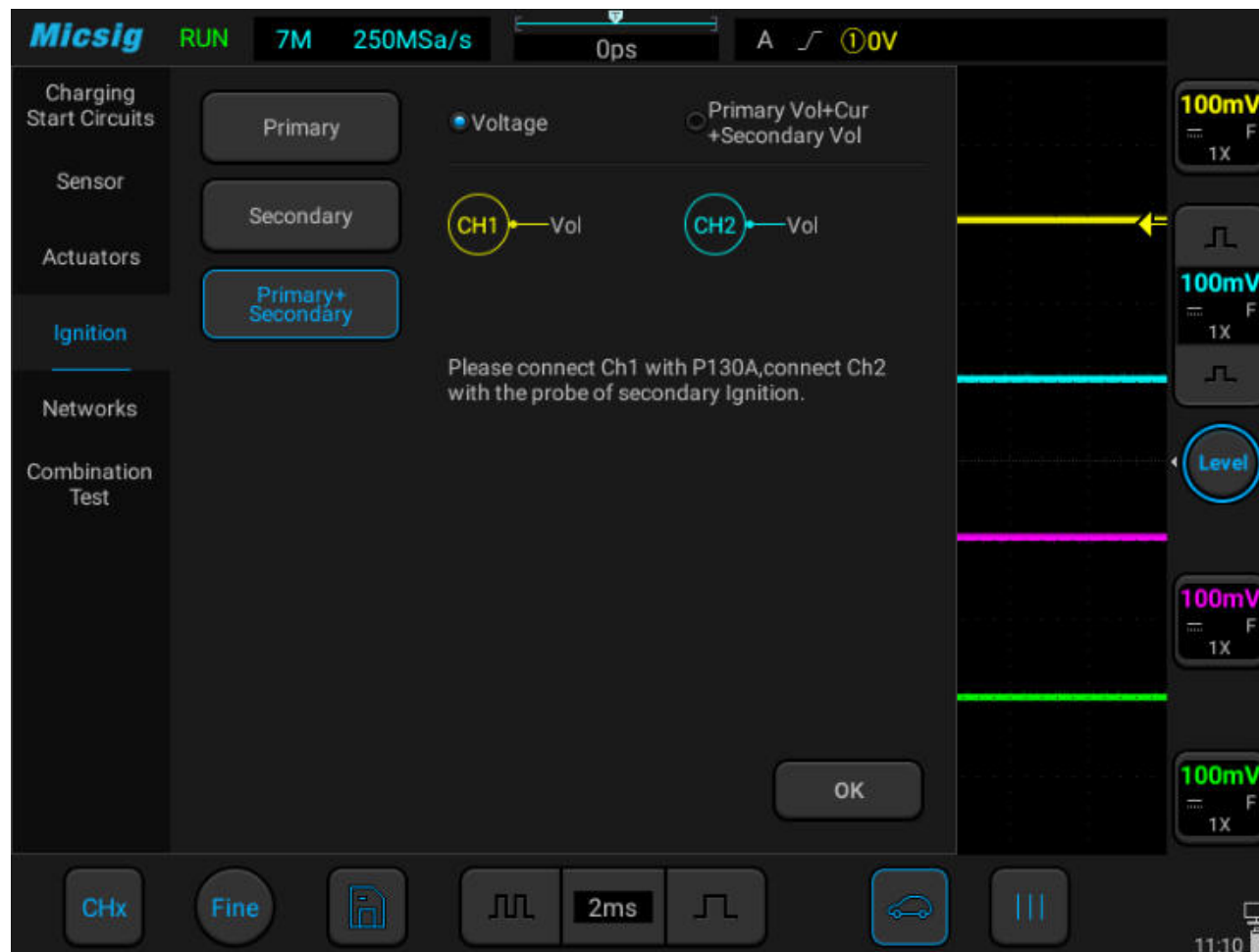
Figure 3-43: Primary + Scondary ignition test
