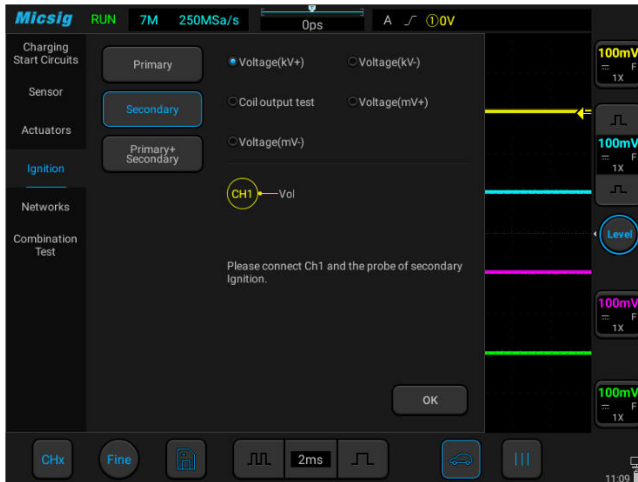
Figure 3-42 Secondary ignition test
