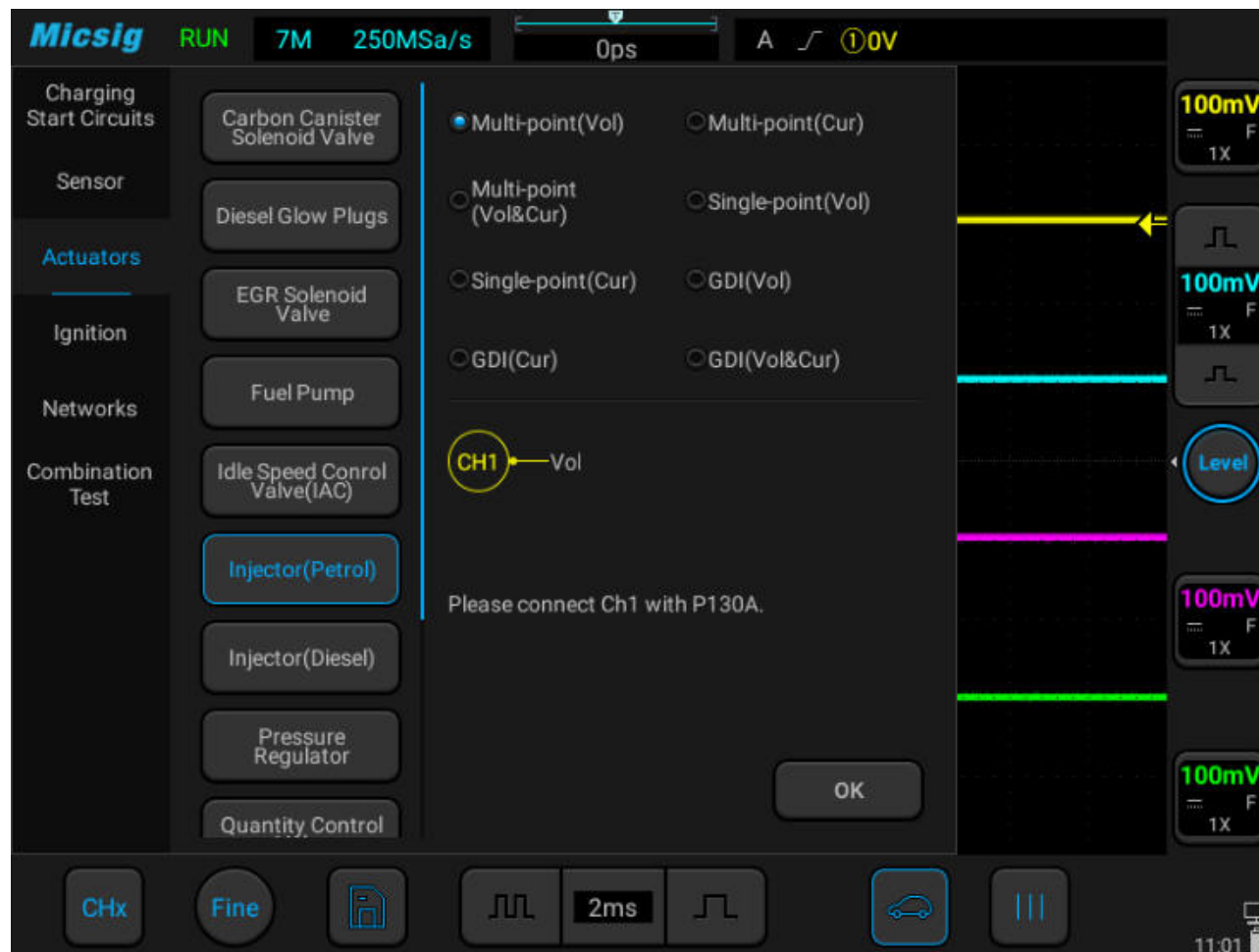
Figure 3-32 Injector (Petrol) Test
