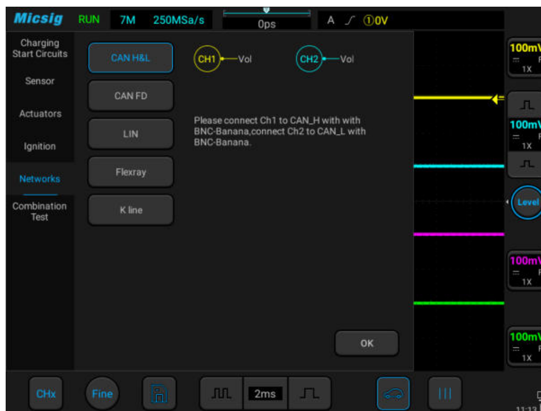
Figure 3-45 CAN BUS Test
