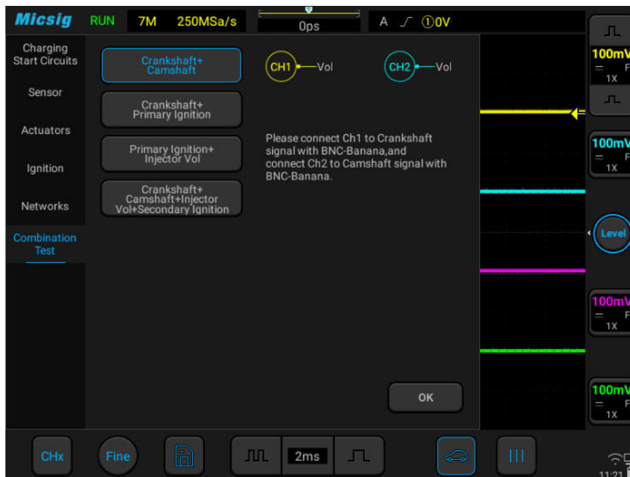
Figure 3-50 Crankshaft + Camshaft Combination Test
