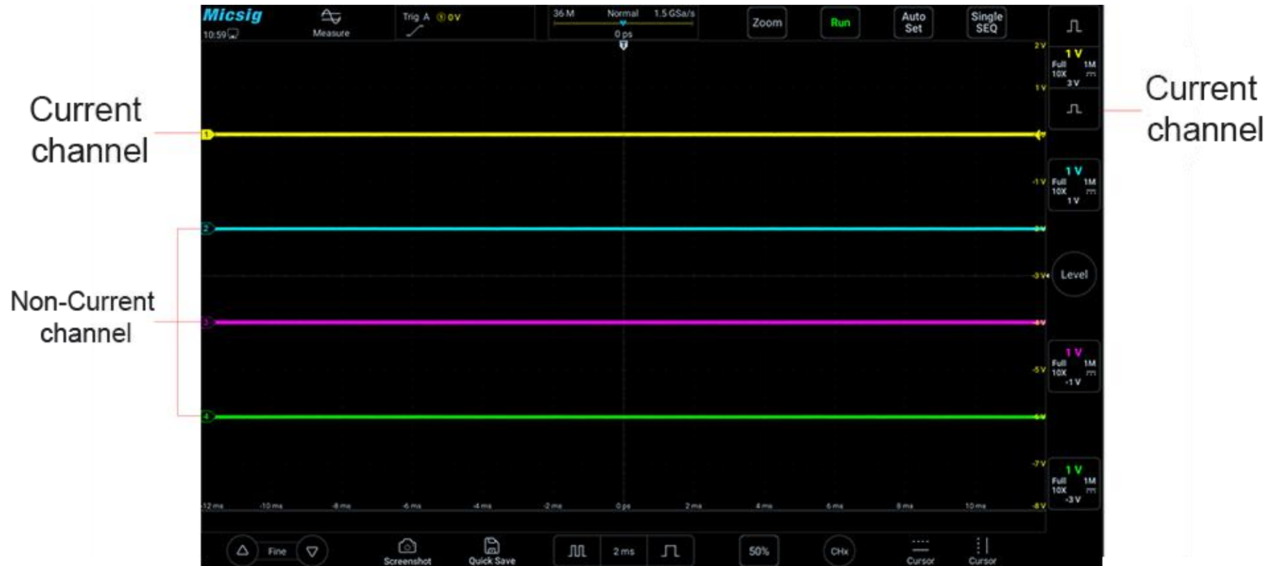
Figure 5-2 Current Channel and Non-Current Channel
