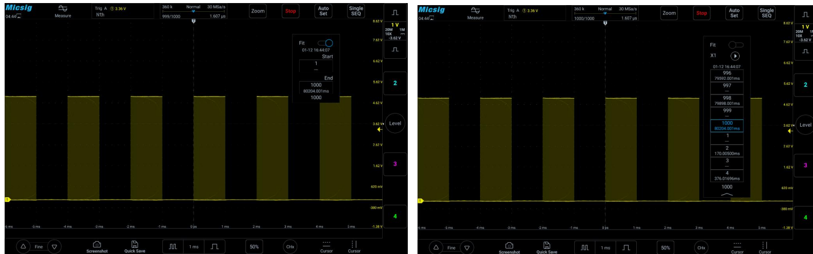
Figure 11-15 View after segment collection is completed
