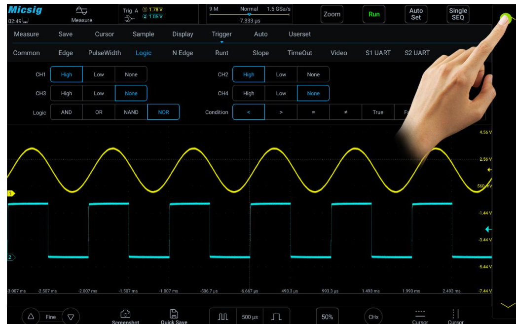
Figure 6-22 Trigger Level Adjustment
