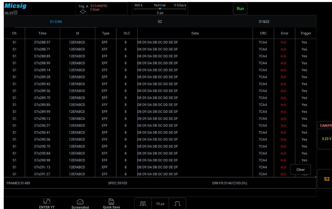
Figure 12-17 CAN bus decode in Text mode
