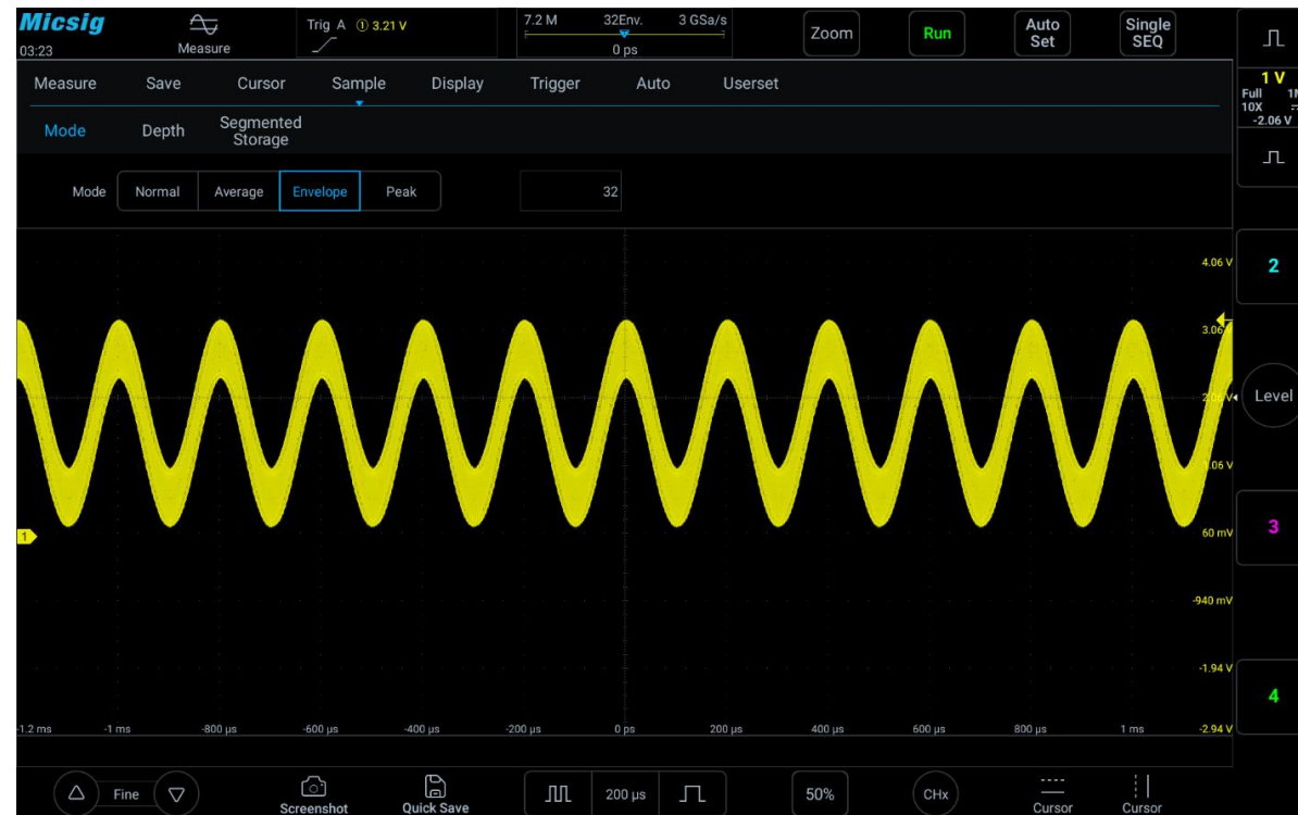
Figure 11-8 Signal in Envelope Sampling Mode (32)
