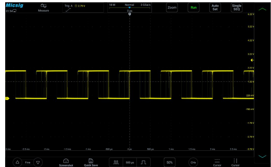
Figure 6-2 Non-Stably Displayed Periodic Signal
