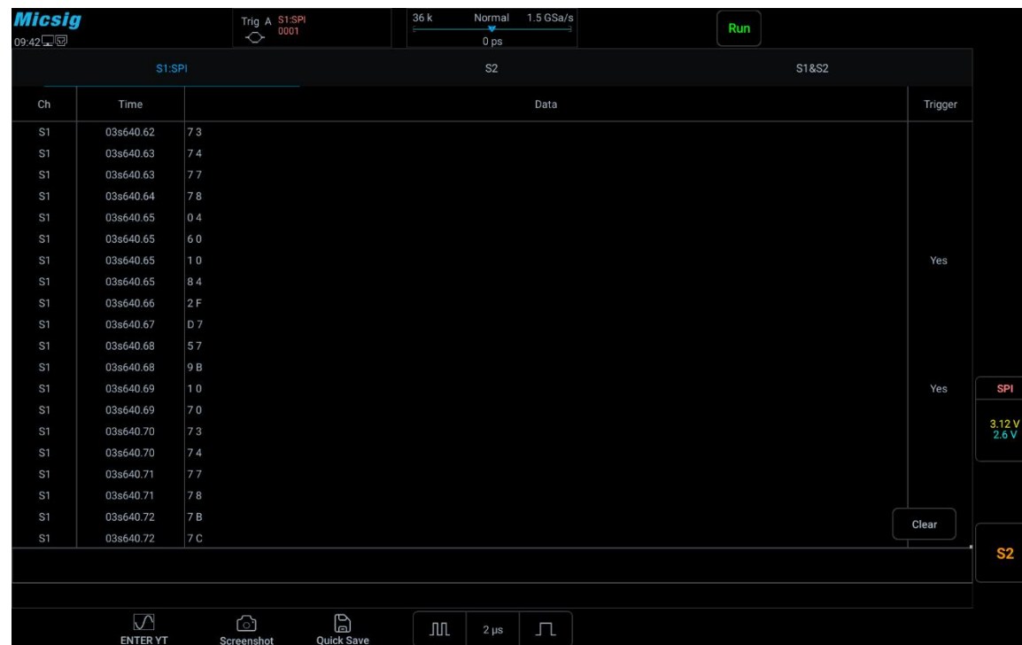
Figure 12-21 SPI Text Interface
