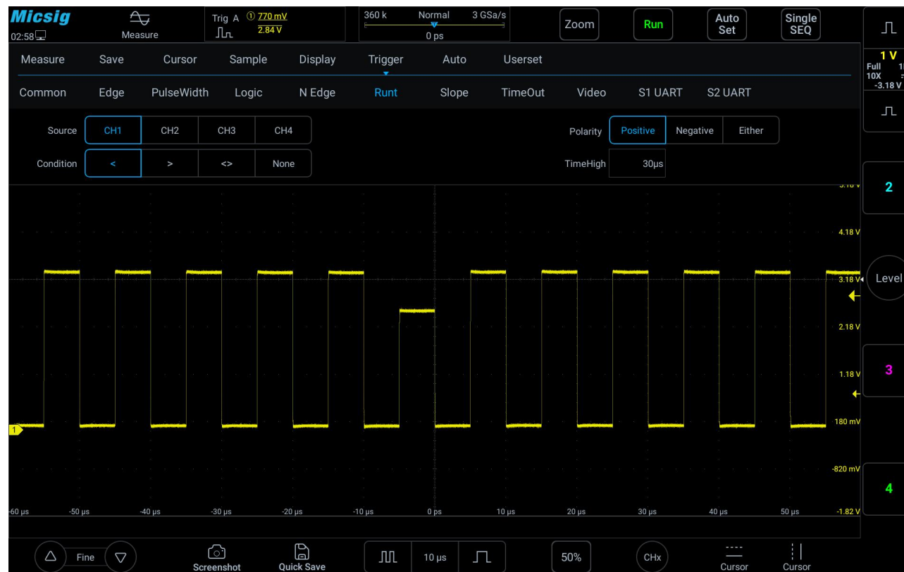
Figure 6-25 Runt Trigger Setting Menu
