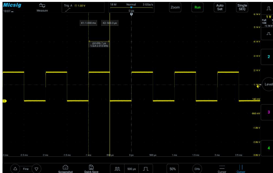
Figure 7-18 Cursor Measurement Pulse Width
