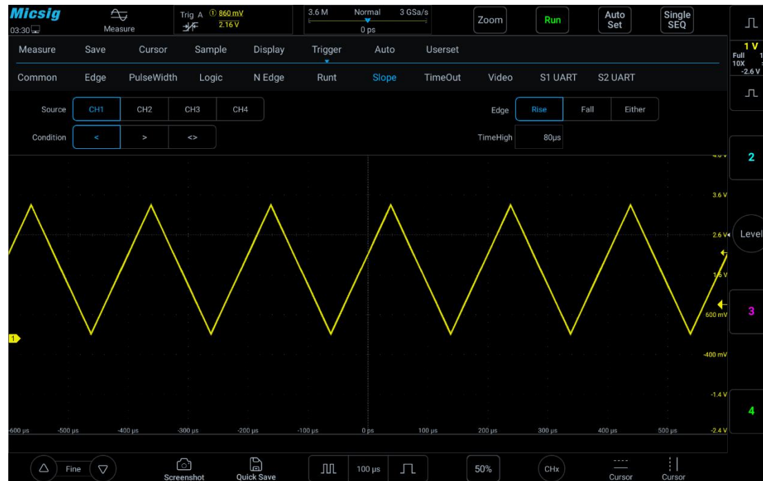
Figure 6-27 Slope Trigger Setting Menu
