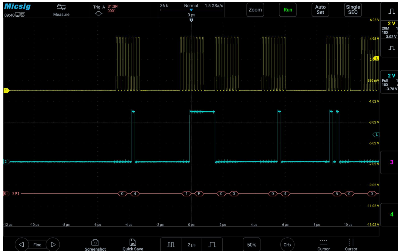
Figure 12-20 SPI bus decode interface
