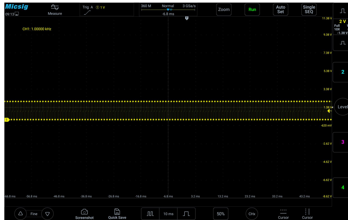
Figure 7-15 Frequency Meter Measurement
