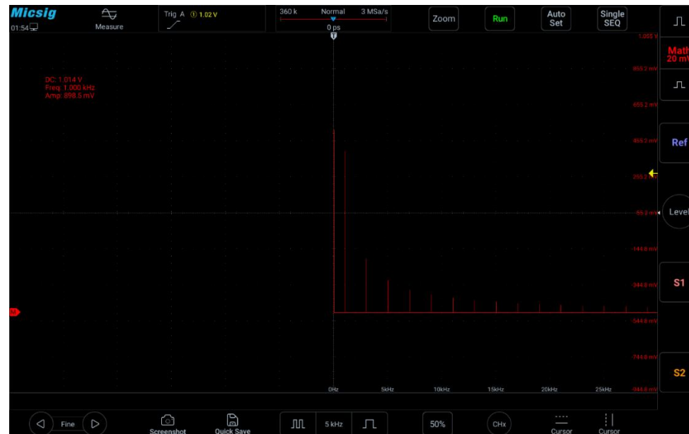
Figure 9-4 Spectrum Amplitude as V-Hz
