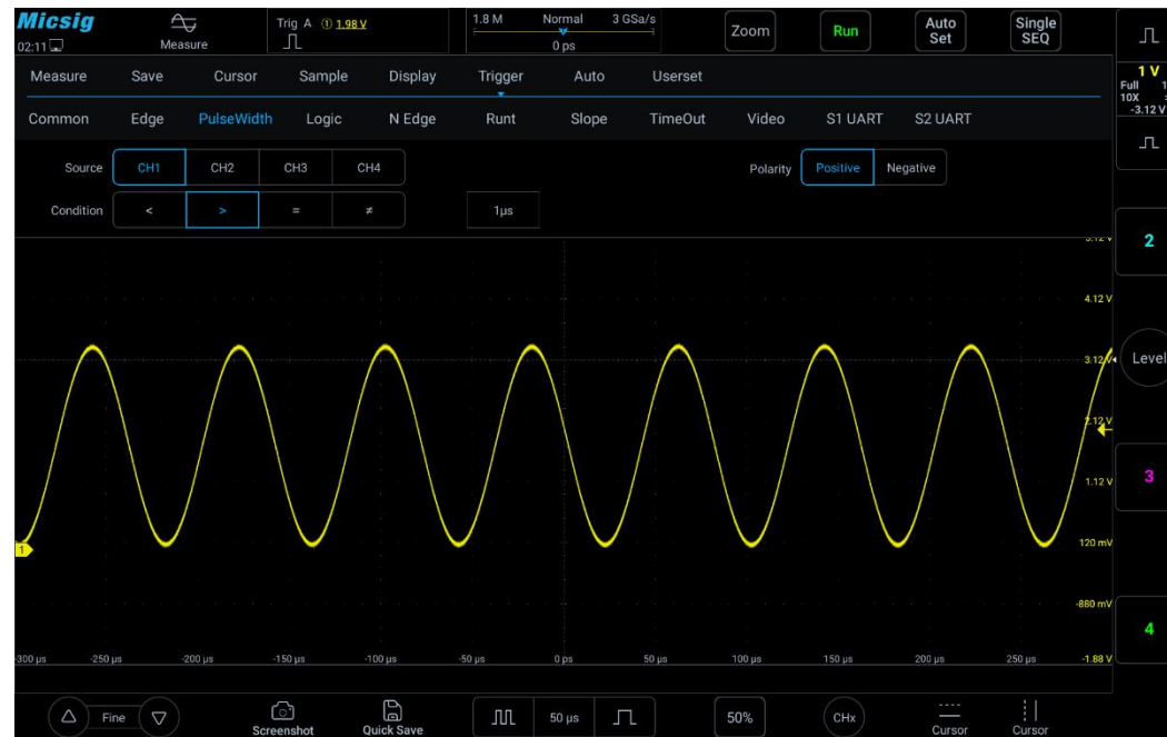
Figure 6-14 Pulse Width Trigger Setting Menu
