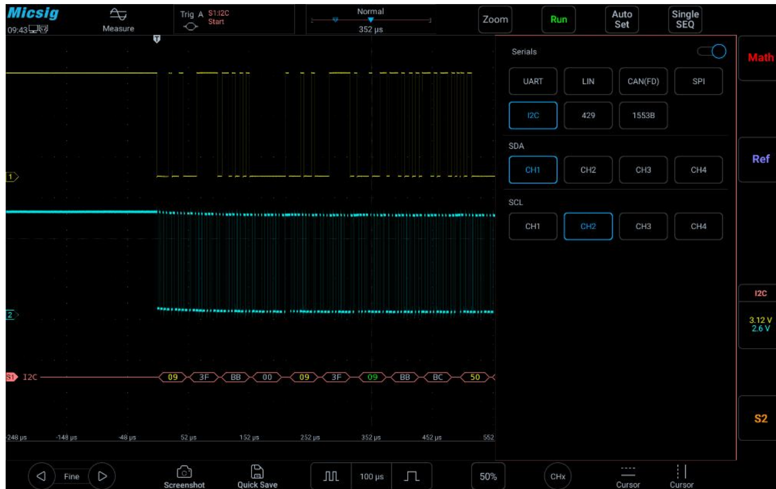
Figure 12-22 I 2 C Bus Configuration Menu
