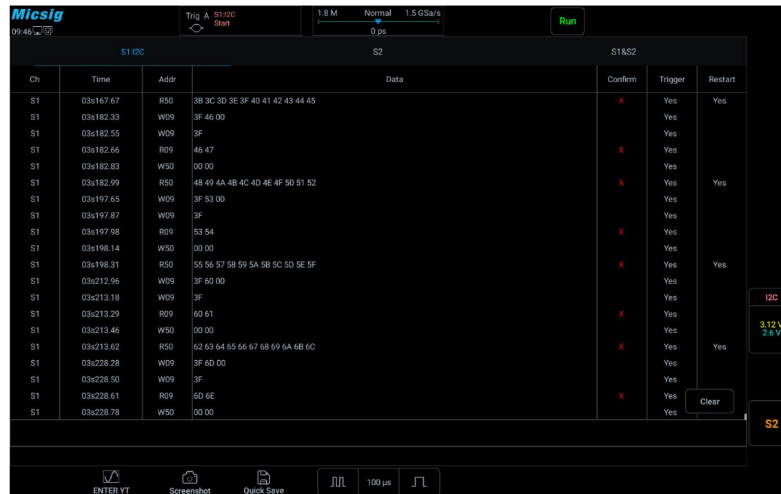
Figure 12-25 I 2 C Text Interface
