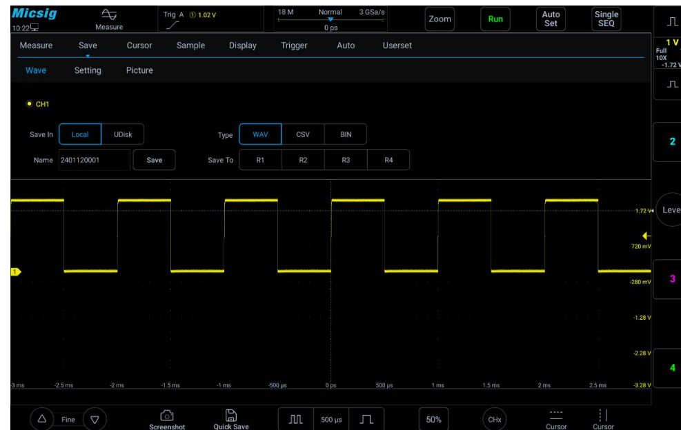
Figure 8-5 Save CH1 Reference Waveform Interface
