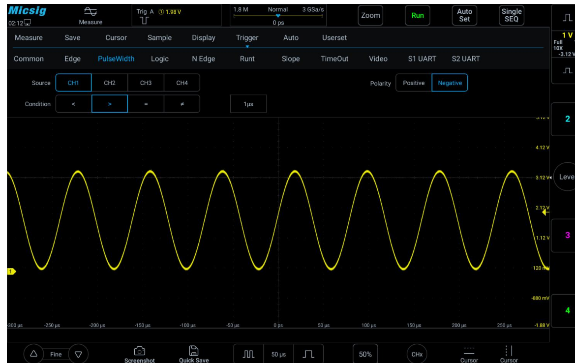
Figure 6-15 Negative Polarity Pulse Level Flip
