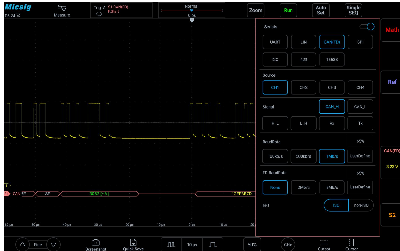
Figure 12-14 CAN / CAN FD Bus Configuration Menu
