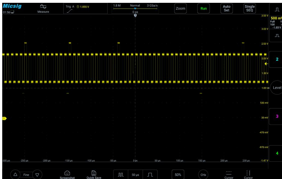
Figure 6-3 Abnormal Signal in Periodic Signals
