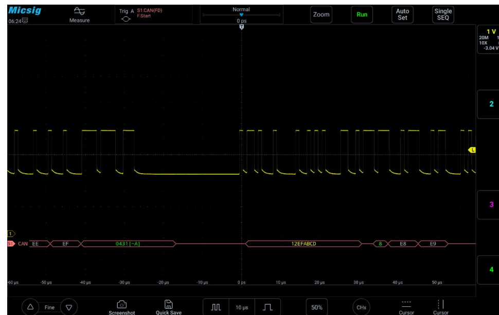
Figure 12-16 CAN bus decode interface
