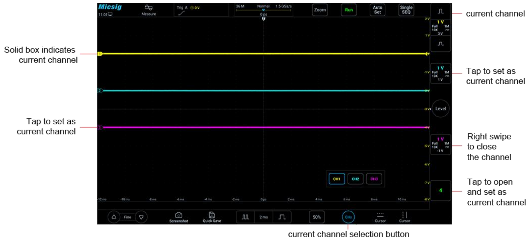
Figure 5-4 Channel Open, Close and Switching
