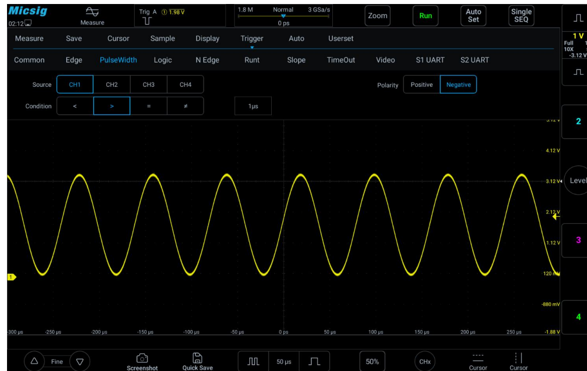
Figure 6-15 Negative Polarity Pulse Level Flip
