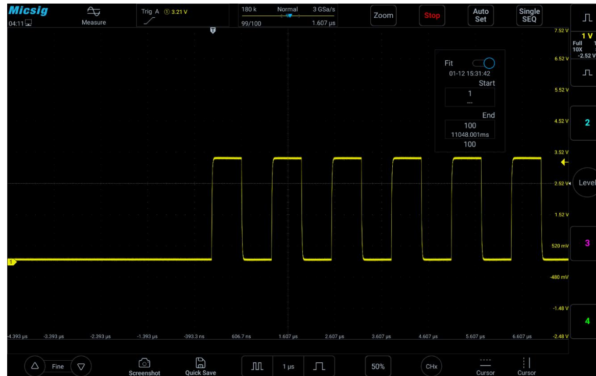
Figure 11-13 Segmented storage fitting view
