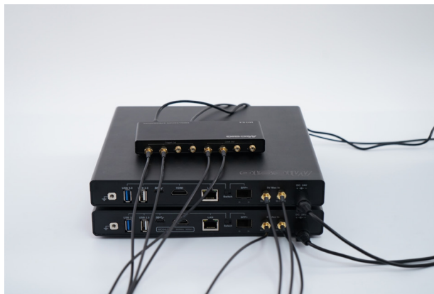
⑥ Connect the synchronizer's Trigger Out to the oscilloscope's Trigger In using an SMA cable.
