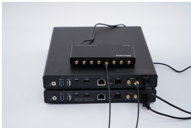
② Connect the synchronizer's Clock Out to the oscilloscope's Clock Input port using an SMA cable.
