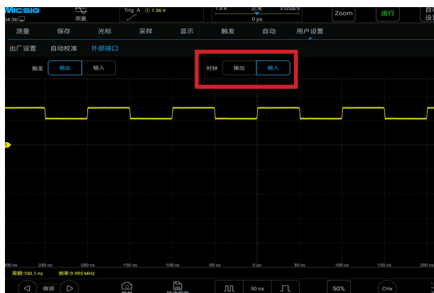
④ Set the oscilloscope to use the external clock input.
