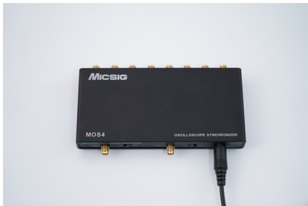
① Power the synchronizer using the supplied power adapter.
