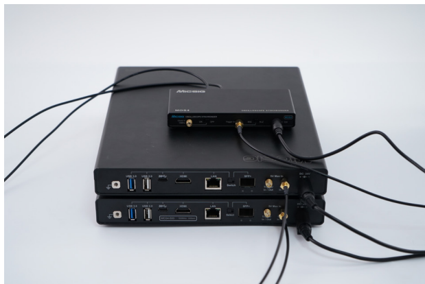
⑤ Connect the external trigger source signal to the synchronizer's Trigger In.
