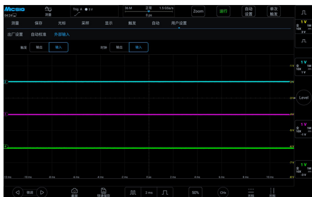
⑦ Set the oscilloscope to use the external trigger input.
