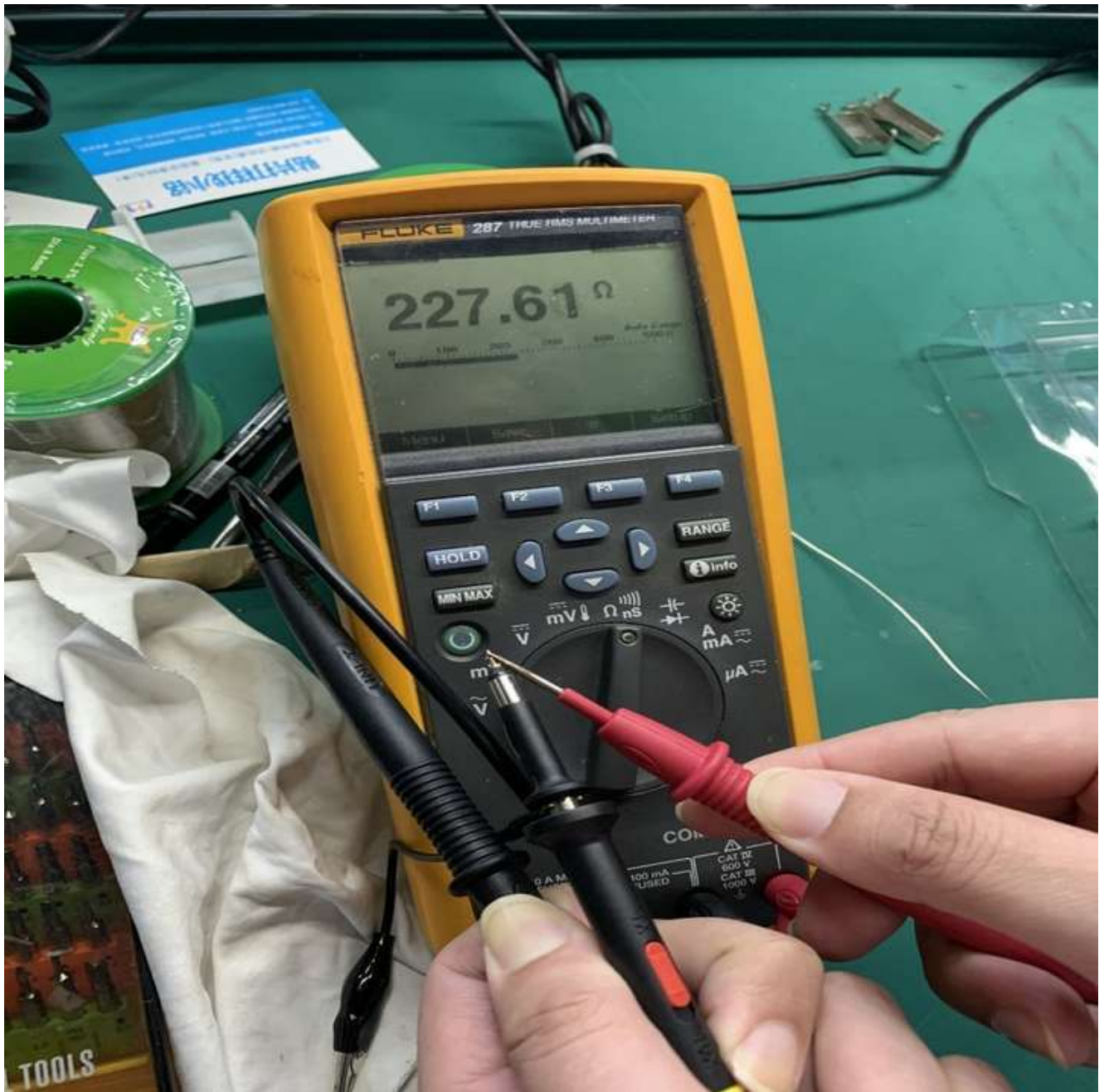
万用表测量探头X1档两端电阻
