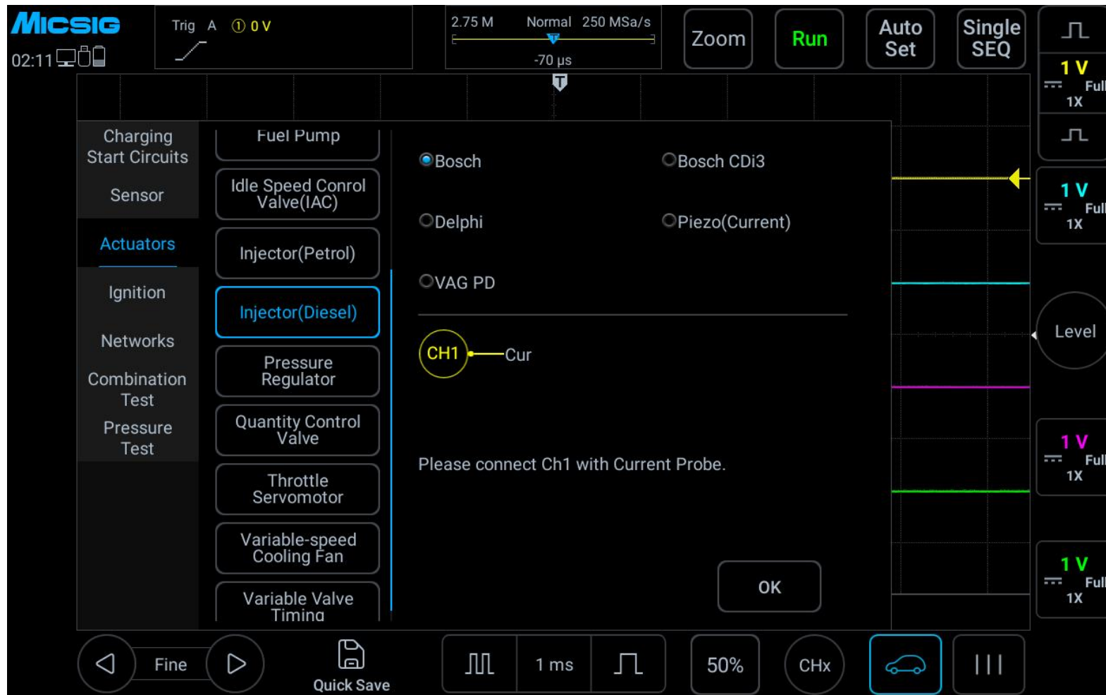
Figure 3-33 injector (diesel engine) test
