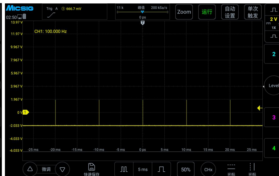
Figure 11-7 Peak Sampling Mode
