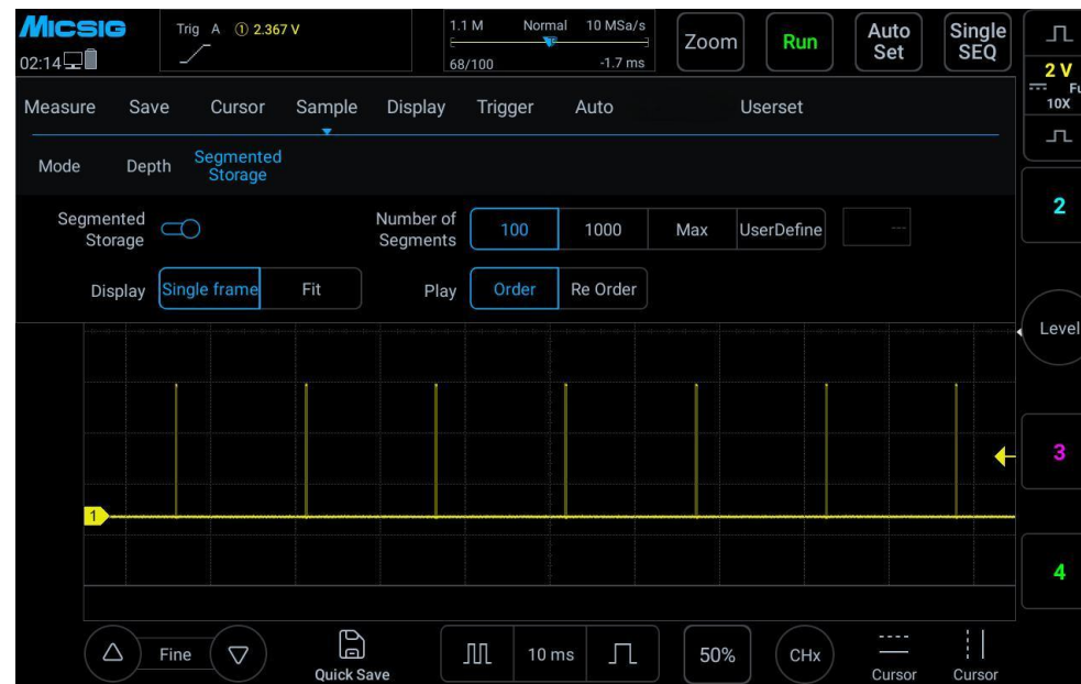
Figure 12-11 Segmented storage waveform acquisition
