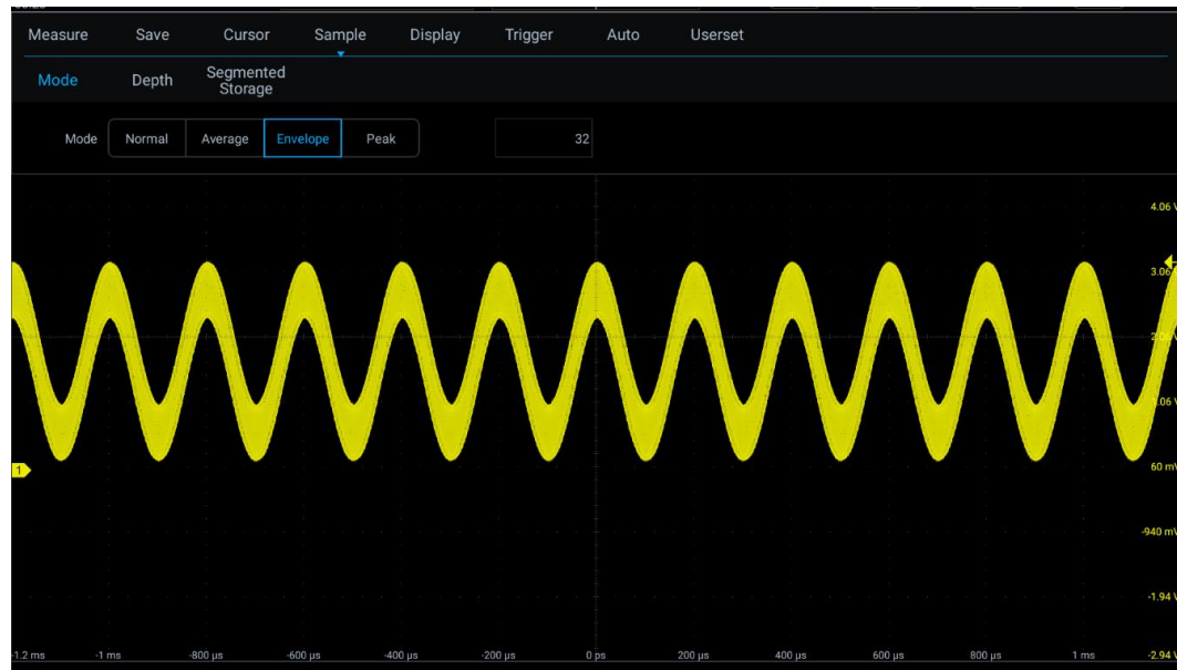
Figure 12-8 The amplitude modulation signal under the envelope sampling mode (32)
