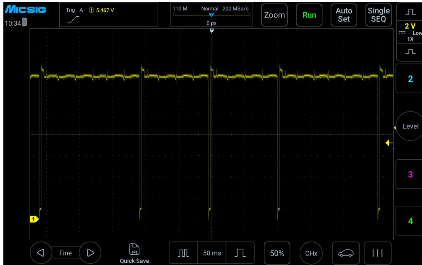
Figure 3-27 Audi A6 Carbon canister solenoid valve signal
