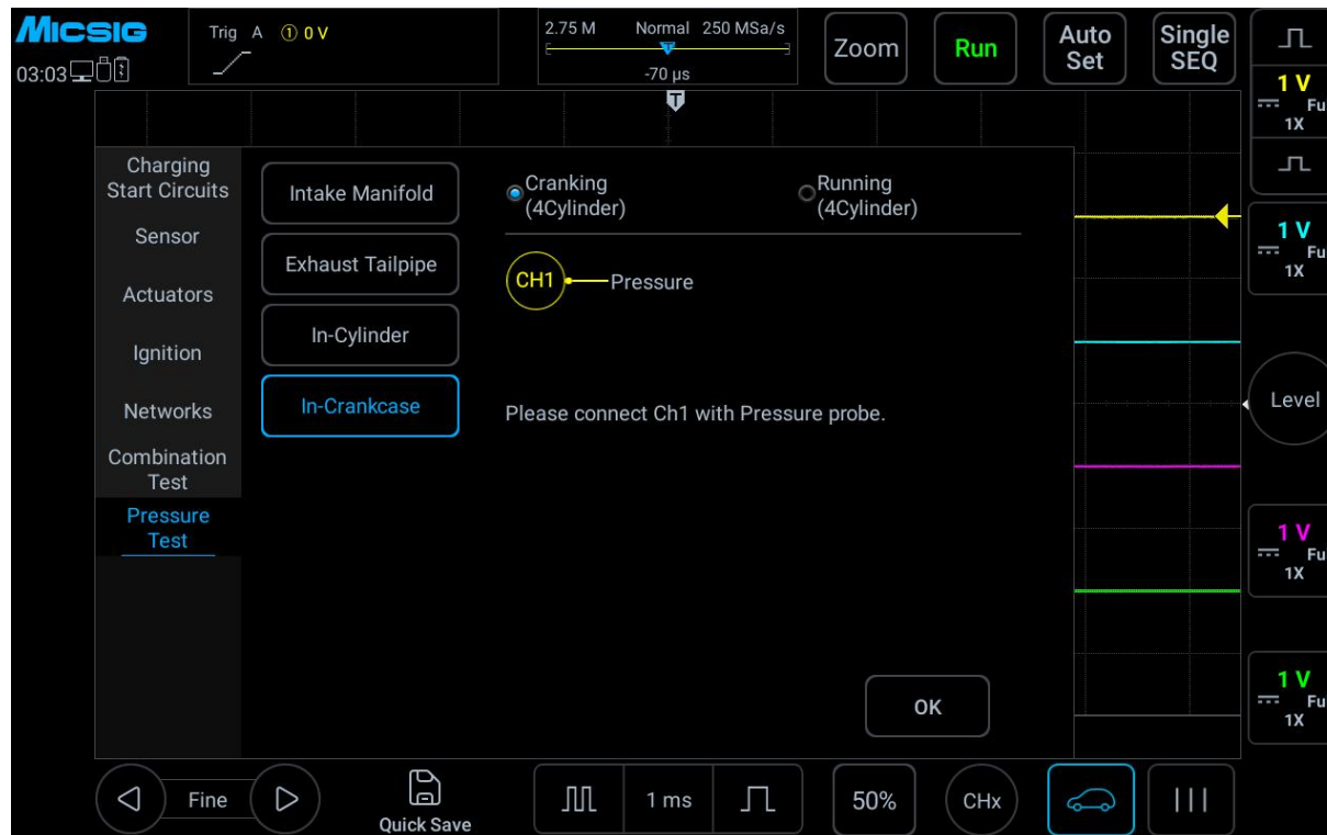
Figure 3-57 In-Crankcase Pressure Test
