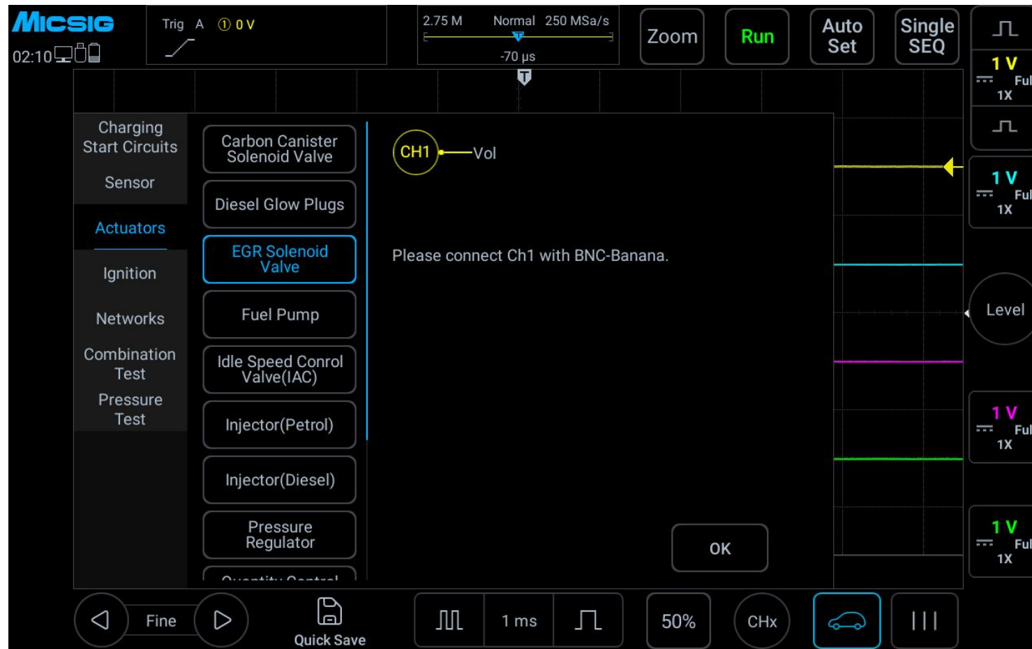
Figure 3-29 EGR solenoid valve test
