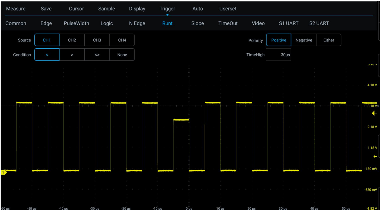
Figure 7-25 Runt Trigger Setting Menu
