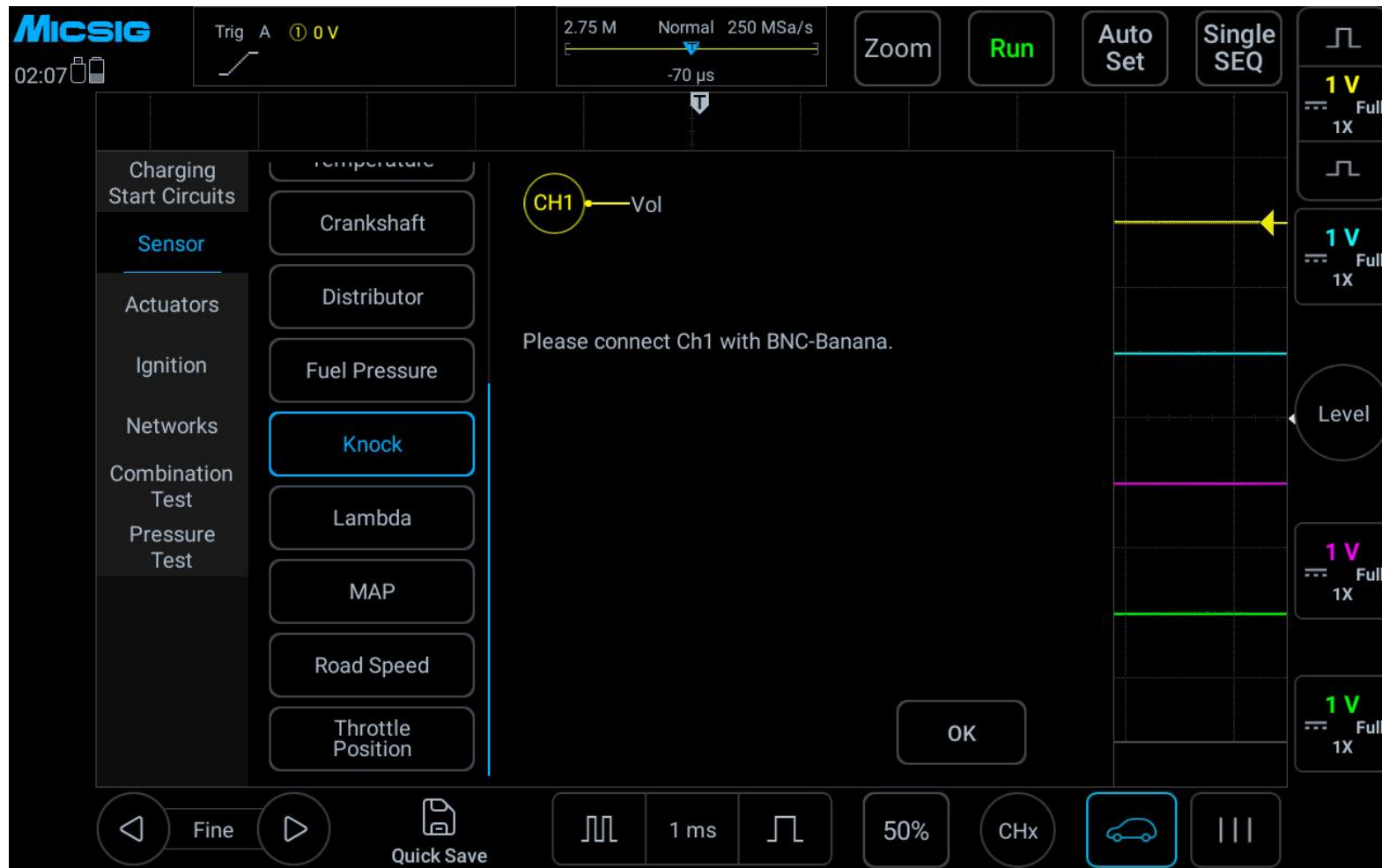
Figure 3-19 Knock Sensor test
