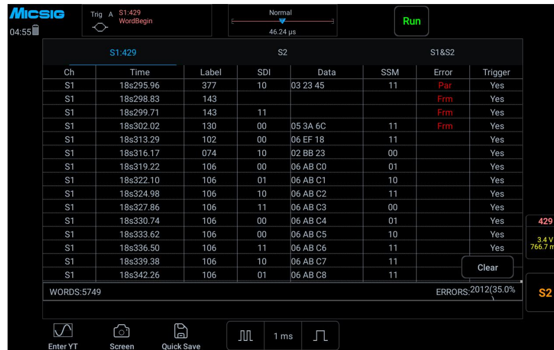
Figure 13-29 ARINC429 Text Interface
