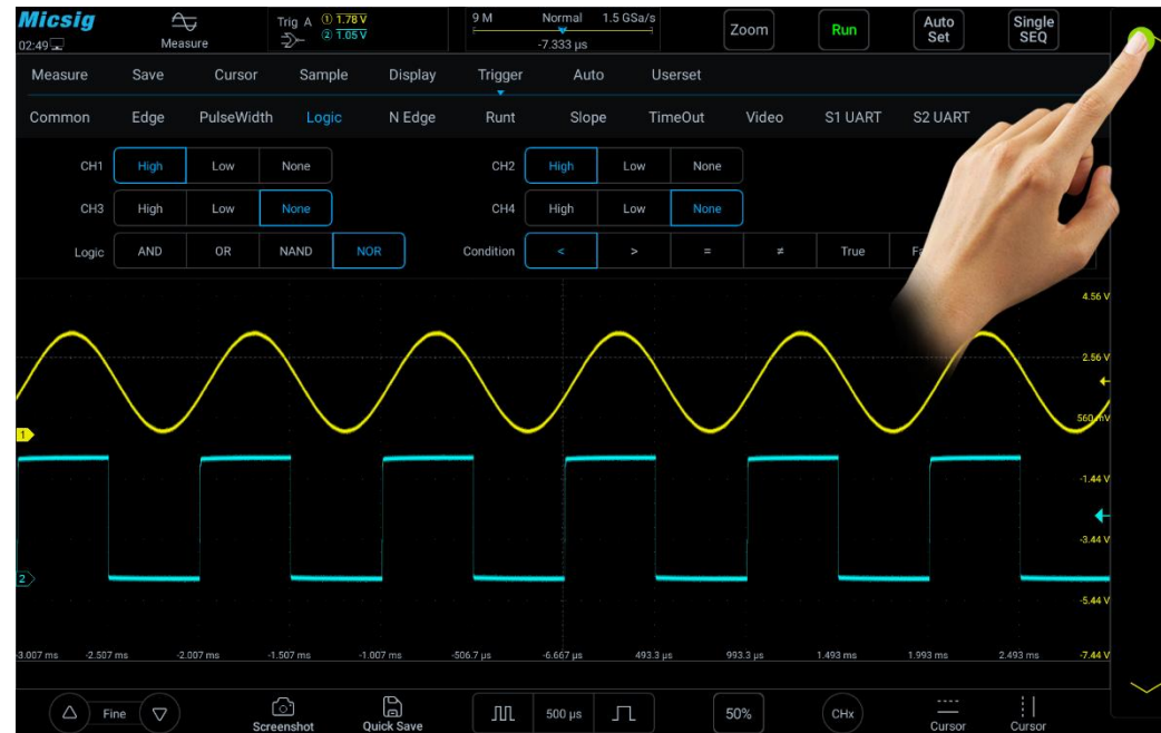
Figure 7-22 Trigger Level Adjustment
