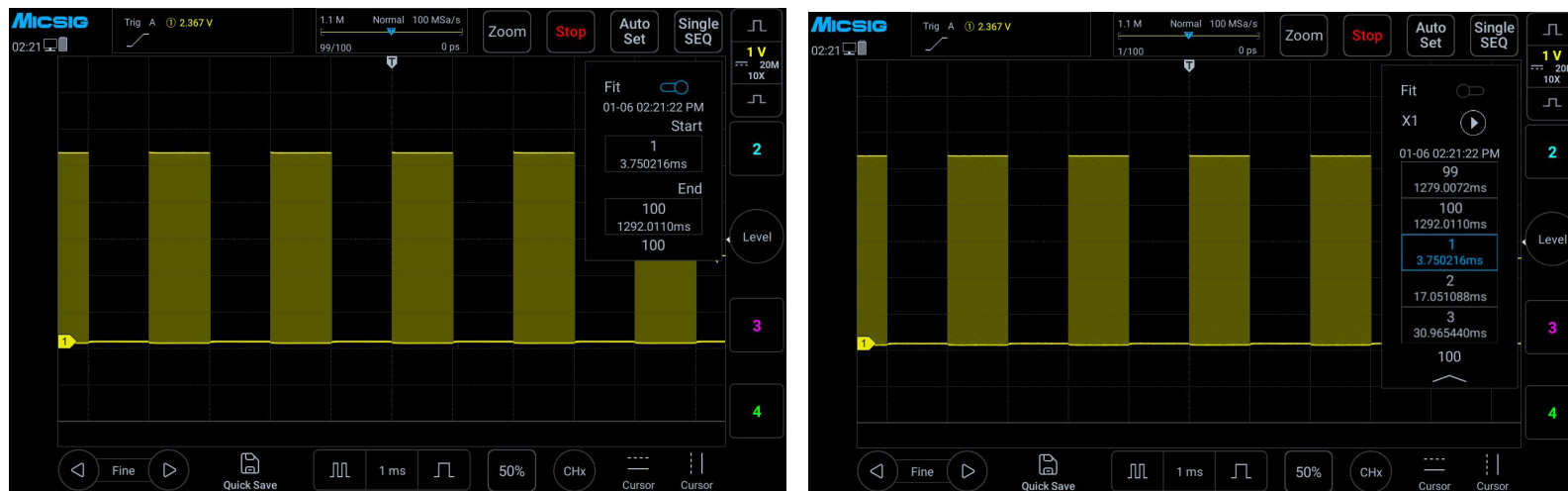
Figure 12-15 View after segment collection is completed
