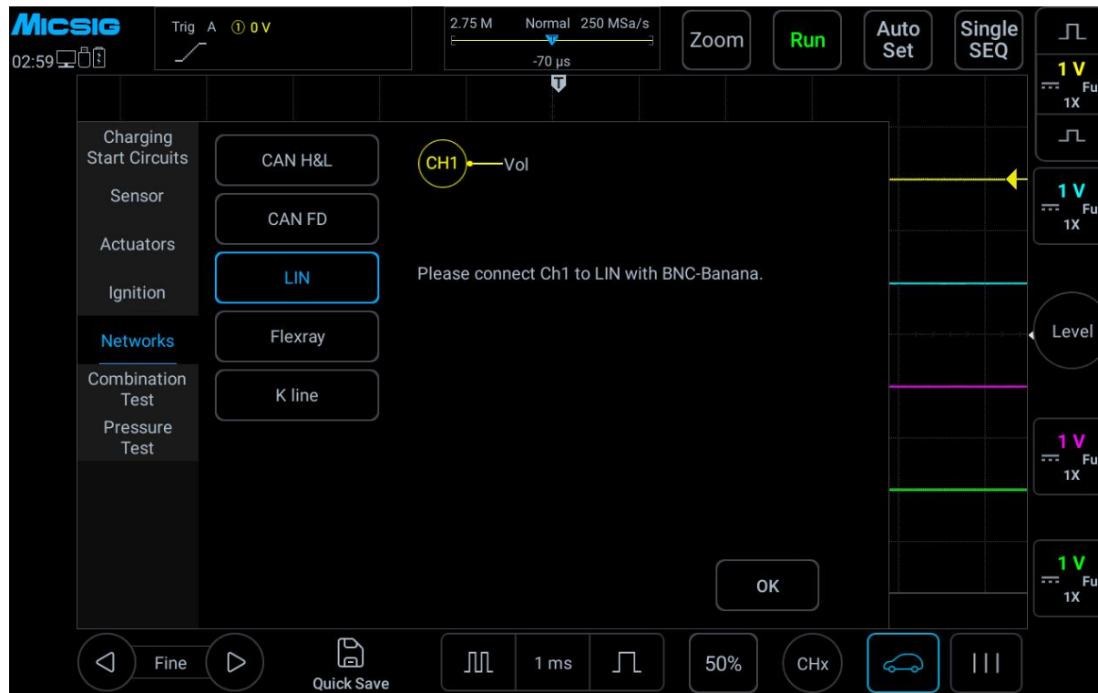
Figure 3-46 Lin bus test
