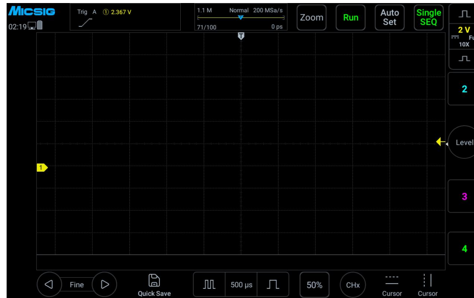
Figure 12-14 Single trigger segmented storage
