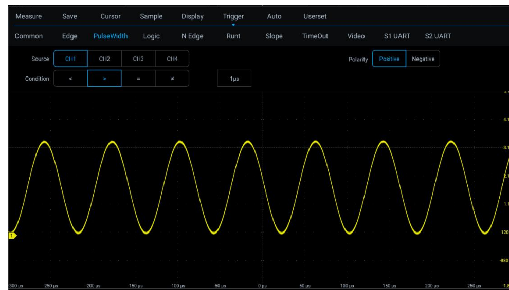
Figure 7-14 Pulse Width Trigger Setting Menu
