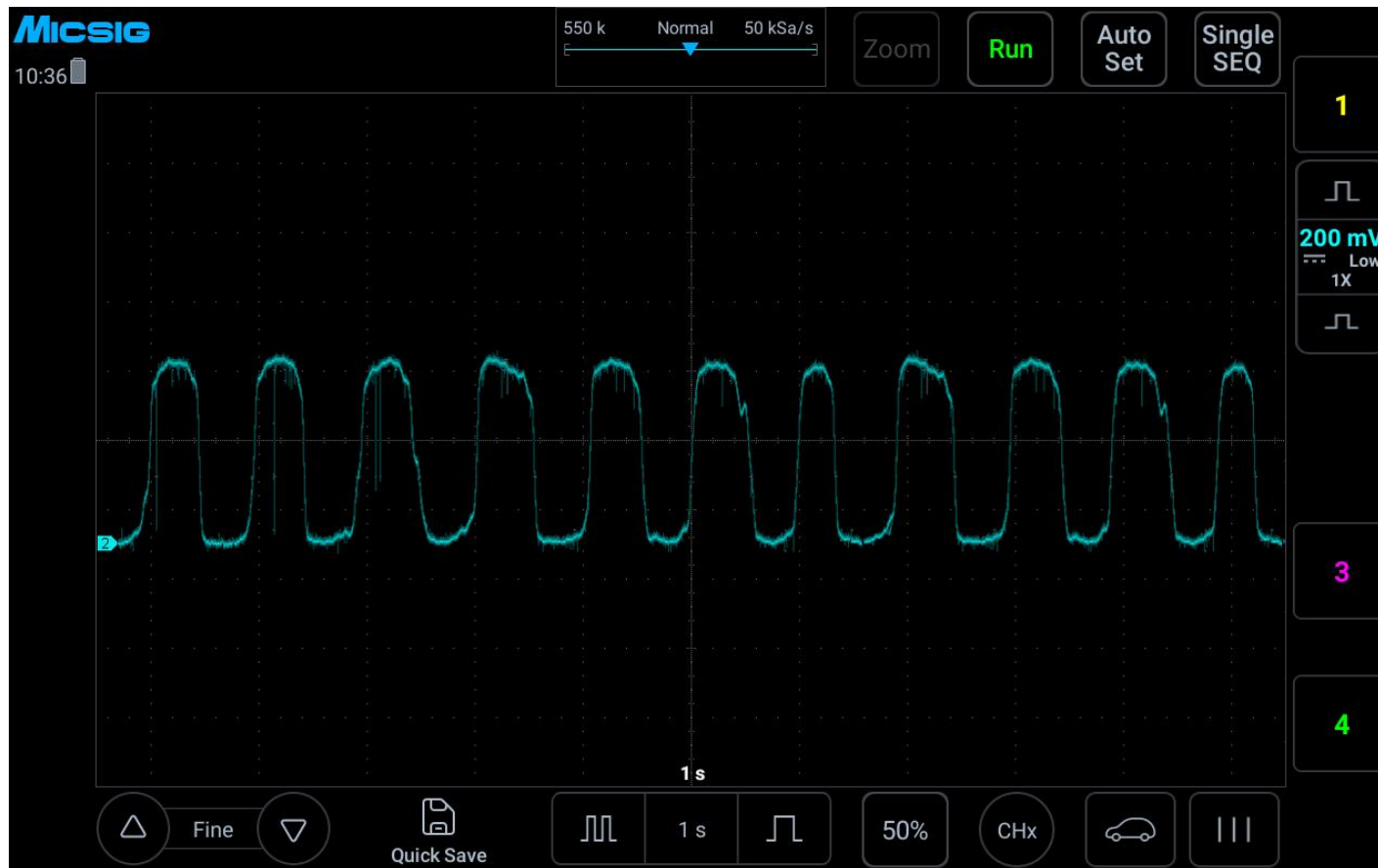
Figure 3-21 Lambda (Oxygen Sensor) diagram
