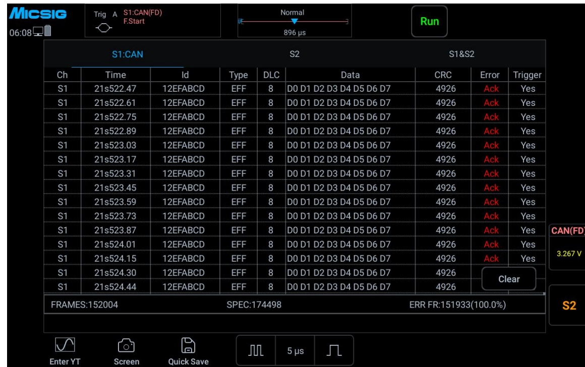
Figure 13-17 CAN bus decode in Text mode
