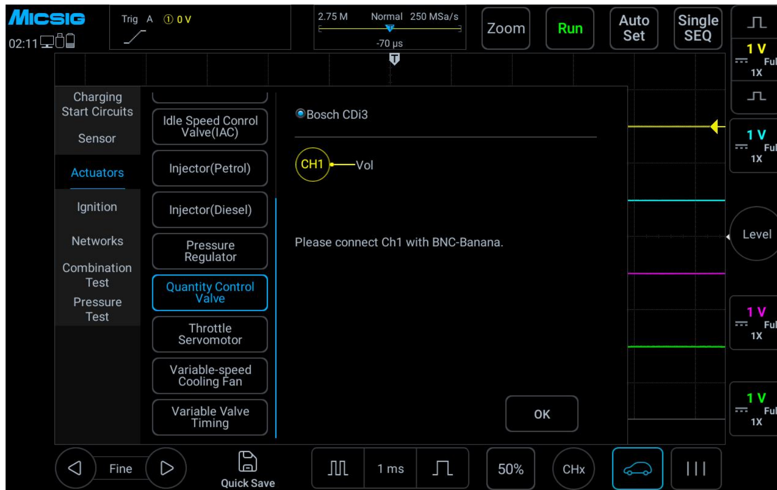
Figure 3-35 Quantity (Flow) control valve test
