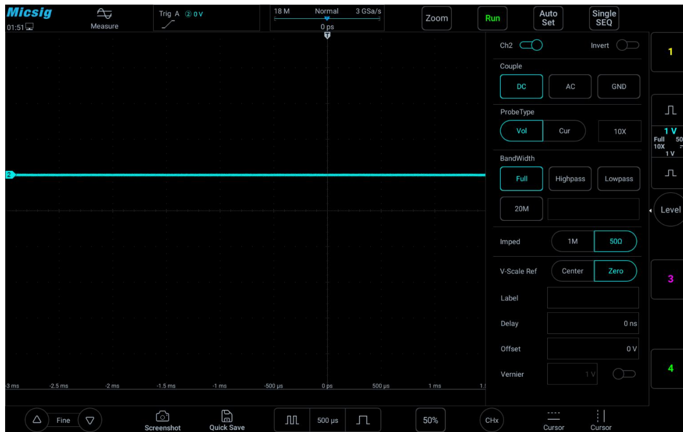
Figure 5-17 Channel input impedance
