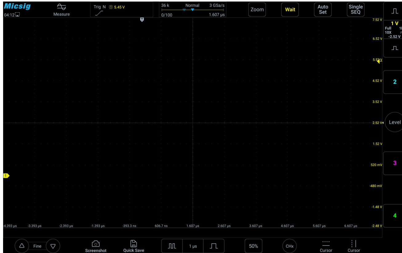
Figure 11-14 Single trigger segmented storage
