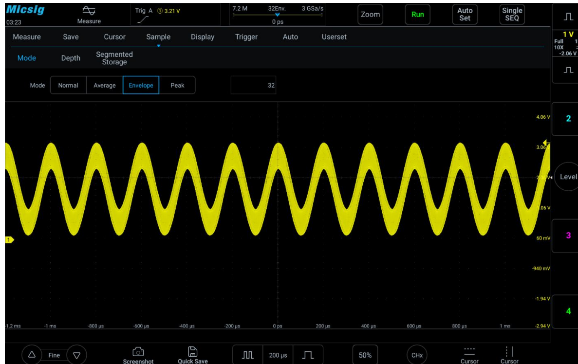
Figure 11-8 Signal in Envelope Sampling Mode (32)
