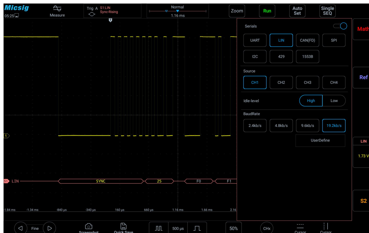
Figure 12-10 LIN Bus Configuration Menu
