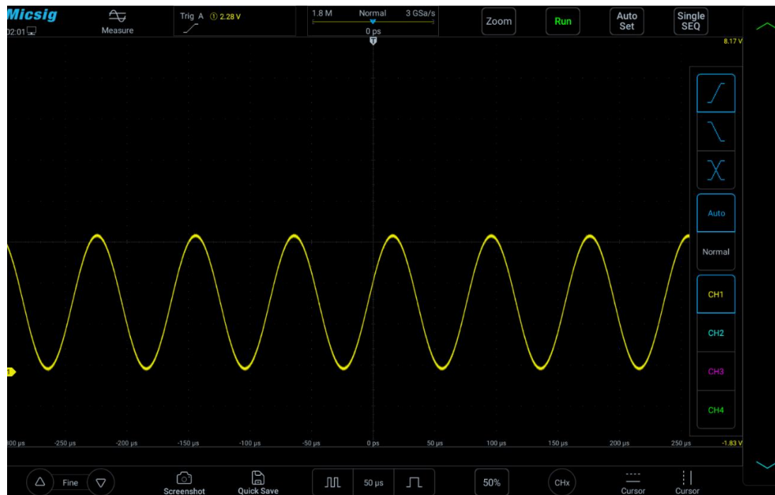
Figure 6-9 Trigger setting shortcut
