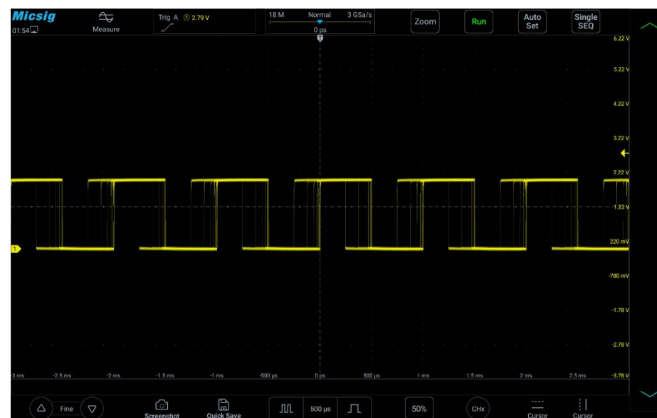
Figure 6-2 Non-Stably Displayed Periodic Signal
