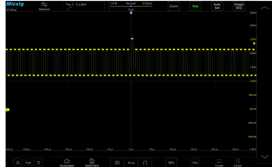
Figure 6-4 Abnormal Signal Captured by Setting Trigger Level
