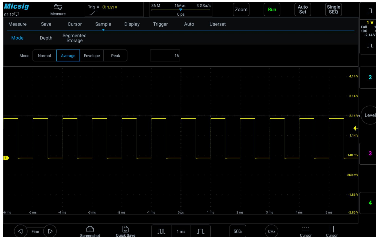
Figure 11-7 Waveform after choosing the average sampling mode, with average number 16
