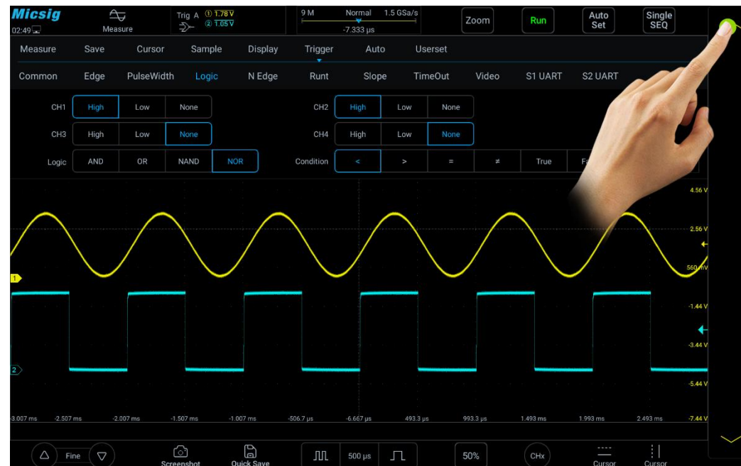
Figure 6-22 Trigger Level Adjustment
