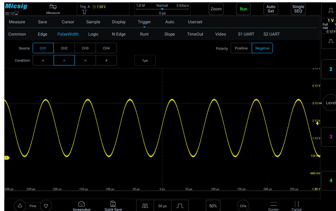
Figure 6-15 Negative Polarity Pulse Level Flip
