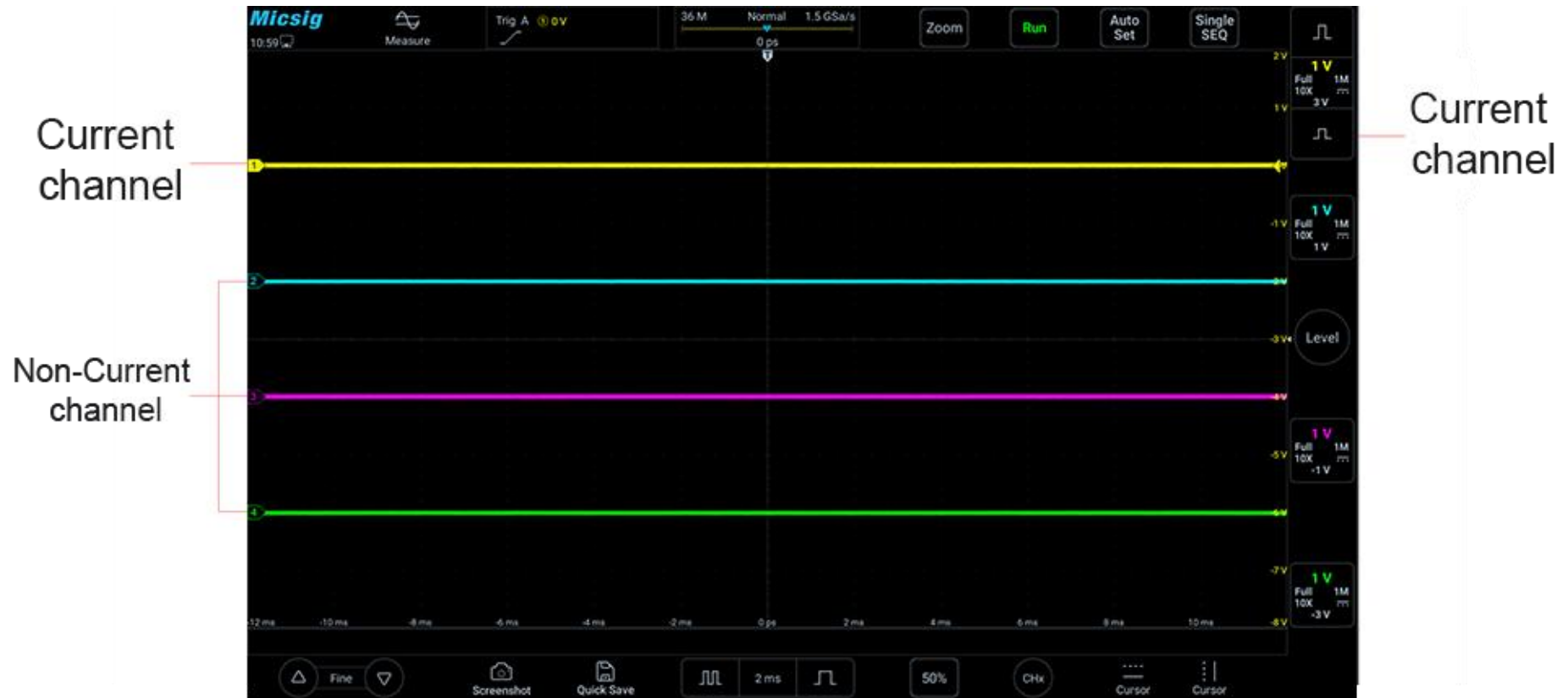
Figure 5-2 Current Channel and Non-Current Channel
