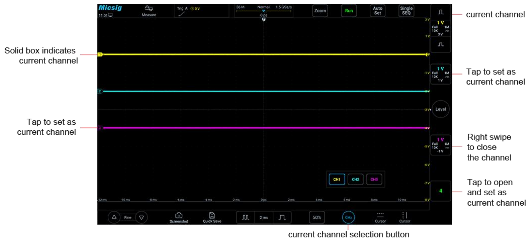
Figure 5-4 Channel Open, Close and Switching
