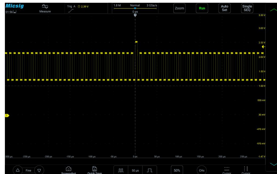
Figure 6-4 Abnormal Signal Captured by Setting Trigger Level
