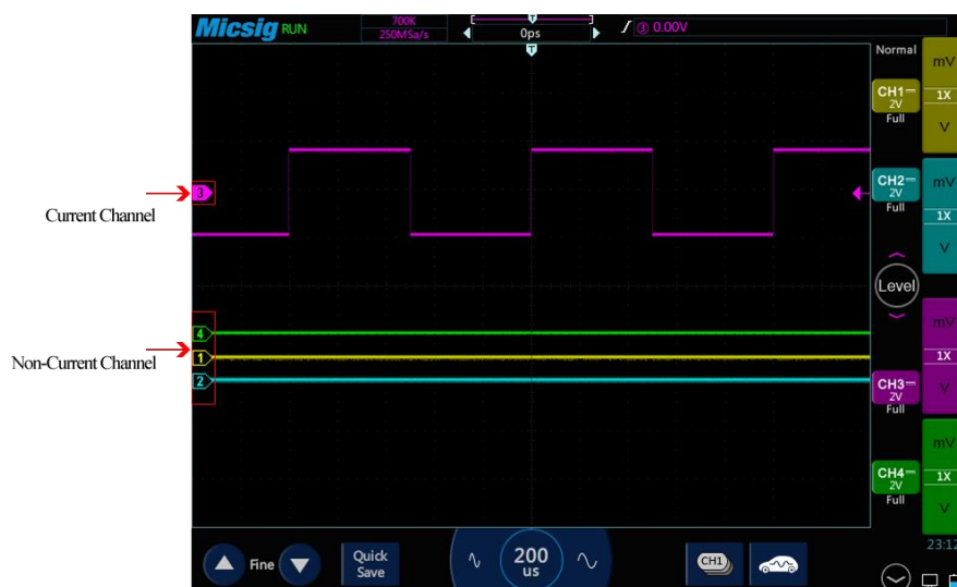
Figure 5-2 Current Channel and Non-Current Channel
