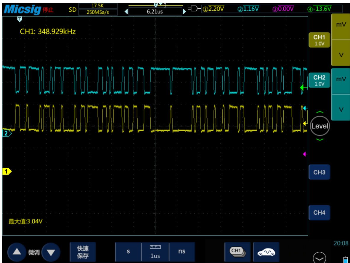
Figure 3-45 CAN BUS Test
