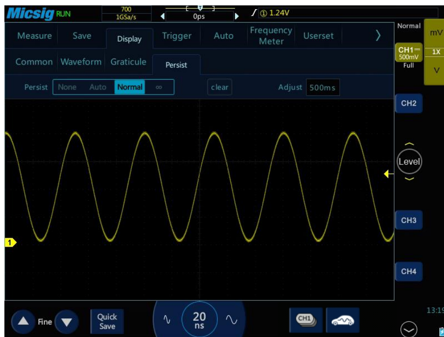
Figure 10-4 20MHz Sine Wave Variable Persistence 500ms
