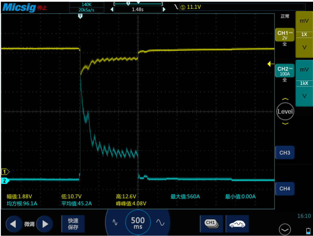
Figure 3-7 Starting voltage and current
