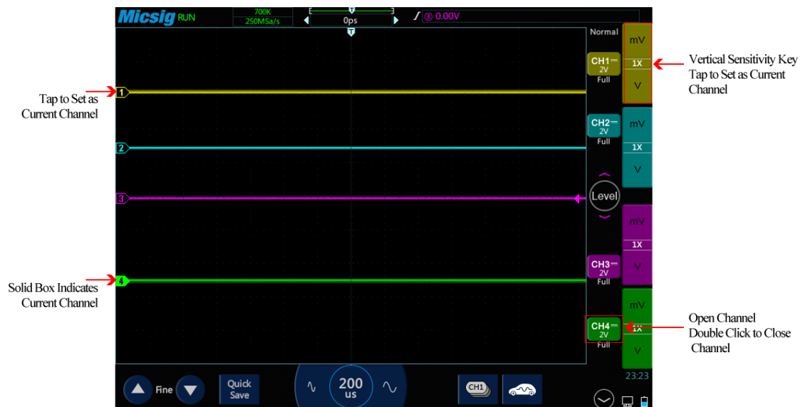
Figure 5-4 Channel Open, Close and Switching
