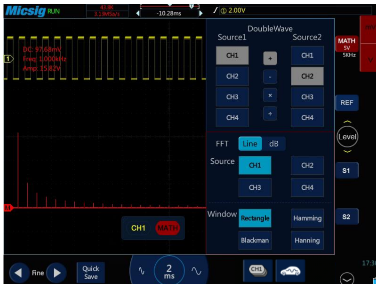
Figure 9-4 Spectrum Amplitude as V-Hz
