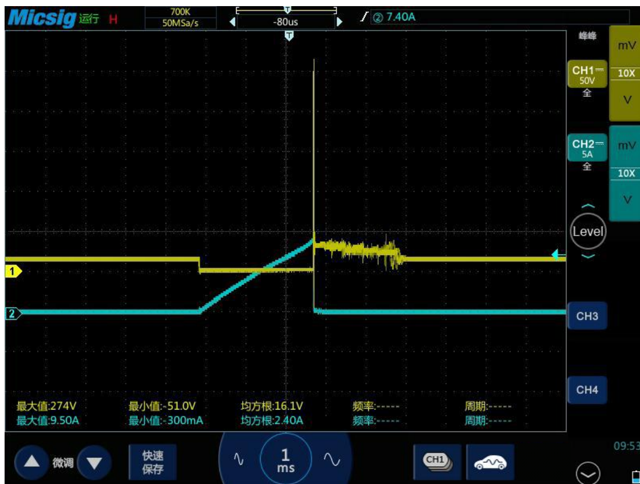
Figure 3-44 BMW 5 Series N20 Primary + Secondary ignition signal
