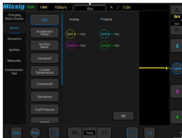
▲ Directly measure the waveform of various Sensors, by comparing with standard waveform, helps user easily find out possible problem.
